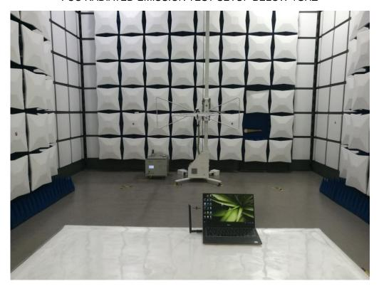
FCC RADIATED EMISSION TEST SETUP ABOVE 1GHZ
