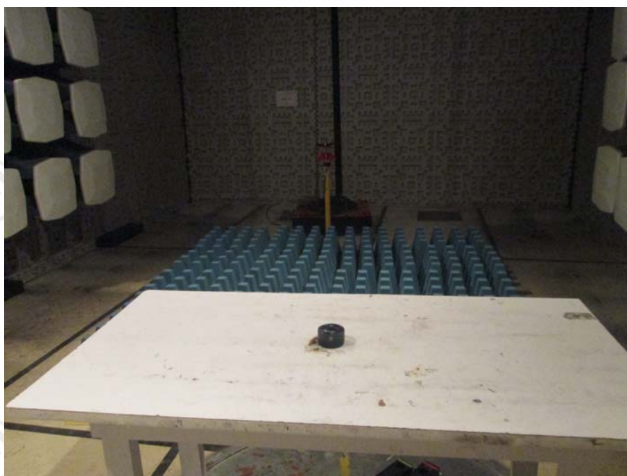
TEST SETUP OF RADIATED EMISSION (above 1GHz)
