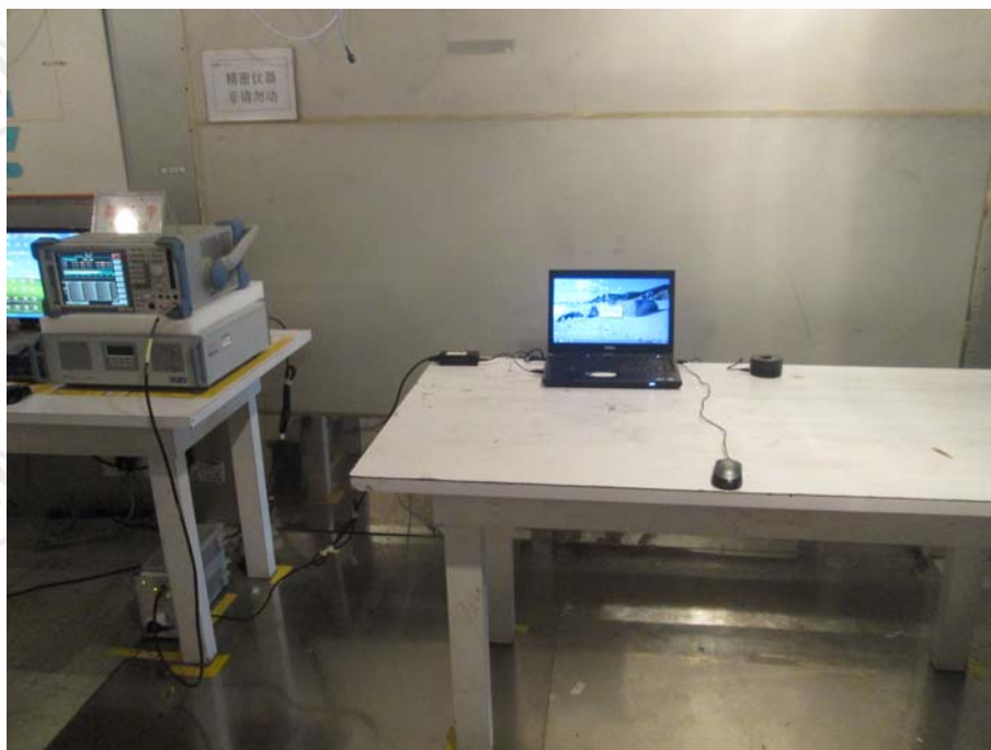
TEST SETUP OF CONDUCTED EMISSION
