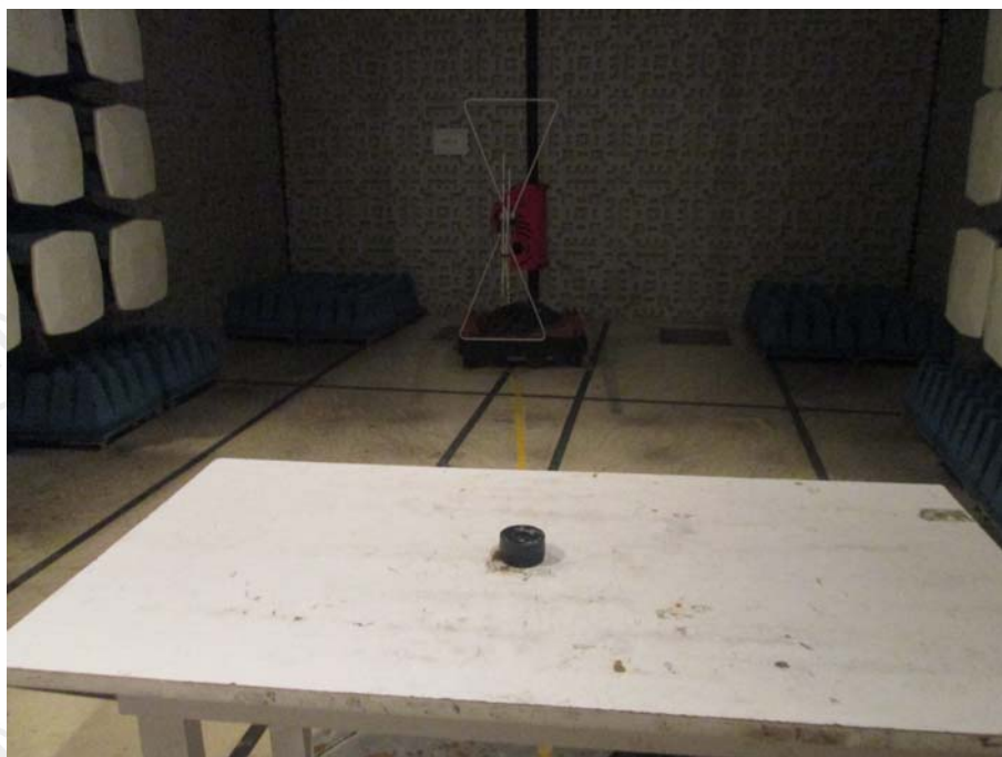
TEST SETUP OF RADIATED EMISSION (30MHz-1GHz)
