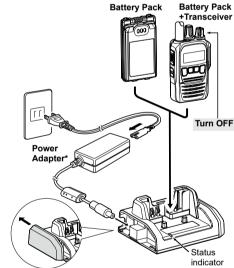
To connect the power adapter to the charger remove the charger's left
