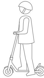
2. Stand with your right foot on the pedal and thrust against the ground with your left foot. When the speed of the scooter is  $\geq 4$  km/h, press the accelerator to start the motor, and keep speeding.
