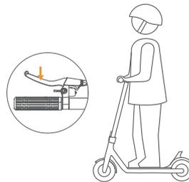
4. When steering or decelerating, release the accelerator and use the brake lever to brake.
