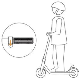
3. During the sliding, keep your balance, place the other foot on the pedal and lightly press the accelerator to move forward.
