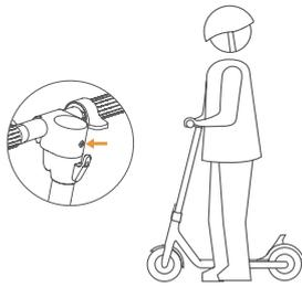
1. Press the switch button to turn on the scooter and check the battery level. If the battery level is too low, please charge it in time.
