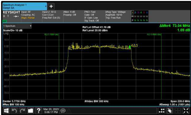
Figure 261 - 802.11ac VHT80 Maximum 6 dB EBW
