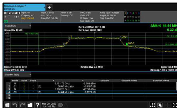
Figure 265 - 802.11ac VHT40 Maximum 99% OBW
