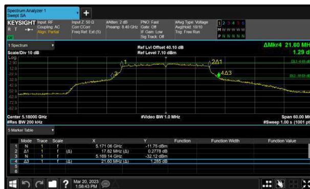
Figure 263 - 802.11ac VHT20 Maximum 99% OBW
