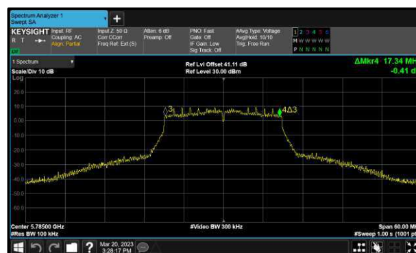
Figure 257 - 802.11ac VHT20 Maximum 6 dB EBW
