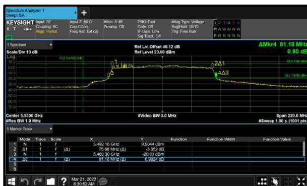
Figure 266 - 802.11ac VHT80 Minimum 99% OBW
