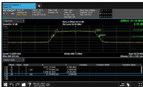
Figure 262 - 802.11ac VHT20 Minimum 99% OBW
