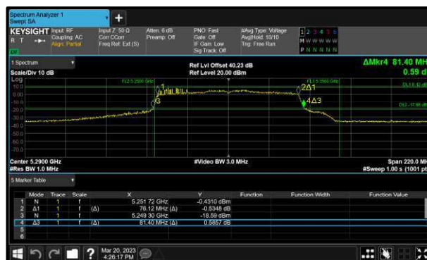
Figure 267 - 802.11ac VHT80 Maximum 99% OBW
