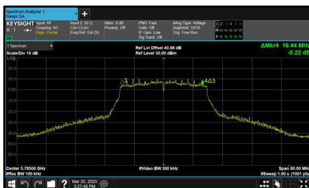
Figure 256 - 802.11ac VHT20 Minimum 6 dB EBW
