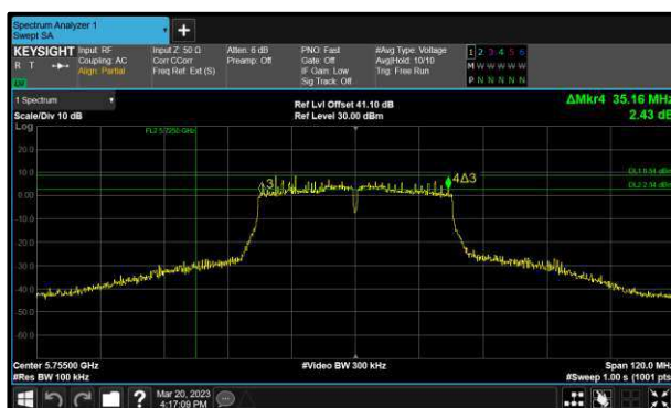
Figure 258 - 802.11ac VHT40 Minimum 6 dB EBW
