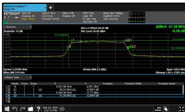
Figure 264 - 802.11ac VHT40 Minimum 99% OBW
