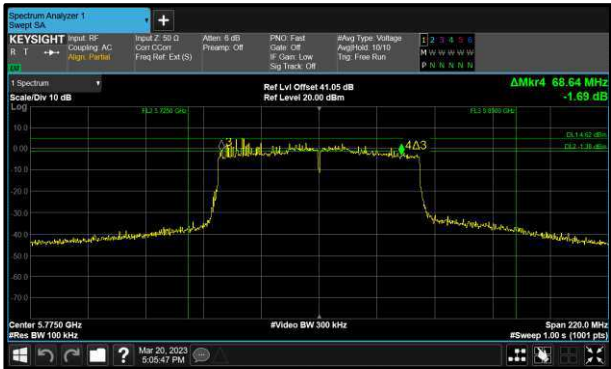
Figure 260 - 802.11ac VHT80 Minimum 6 dB EBW
