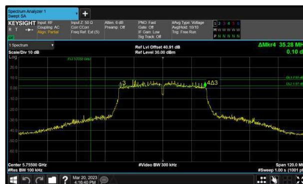
Figure 259 - 802.11ac VHT40 Maximum 6 dB EBW
