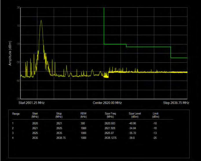
Band38 16QAM BW=15MHz Channel=38175 RB Size=1 Position=#Max Extended
