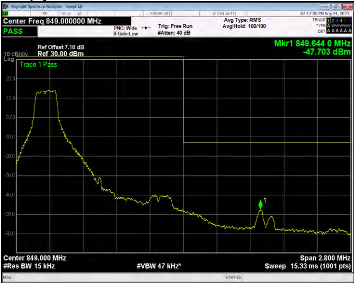
Band26(824-849) QPSK BW=1.4MHz Channel=27033 RB Size=1 Position=#Max Extended
