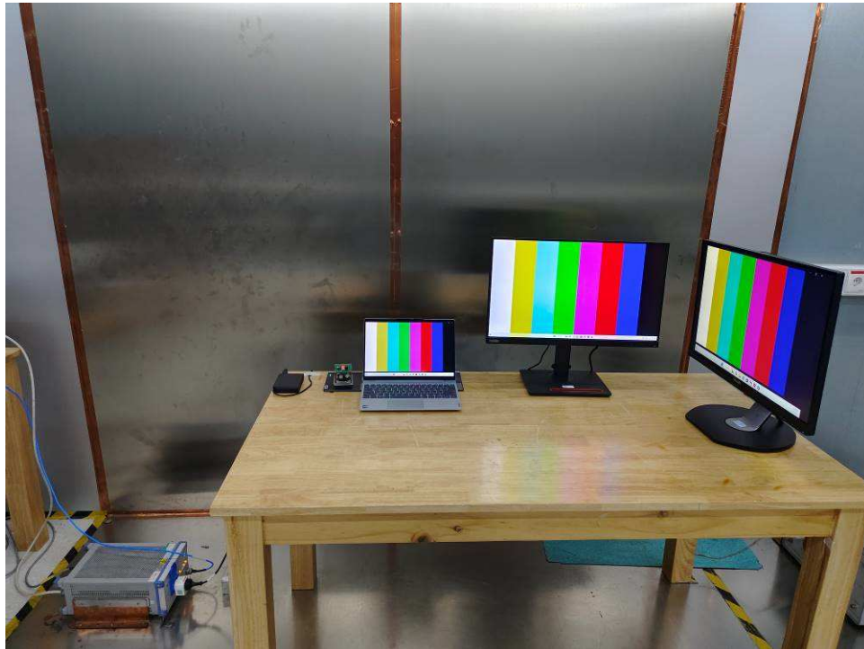
Photograph 1: Set-up for Conducted Emission on AC Mains
