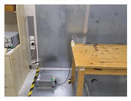
Radiated Emissions From 30MHz-1000MHz
