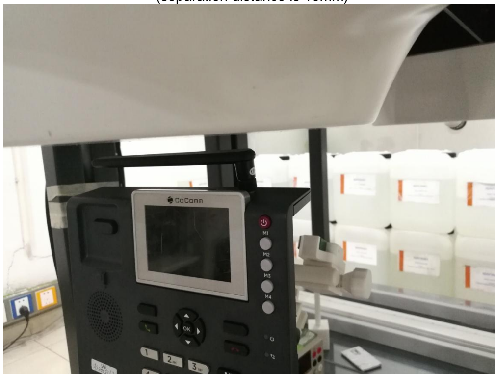
The antennal parallel with the top of device (separation distance is 10mm)
