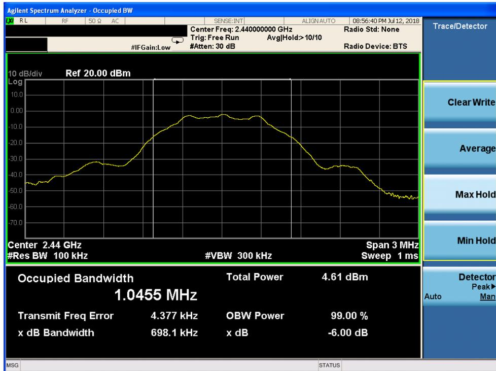
6dB Bandwidth plot on channel 39
