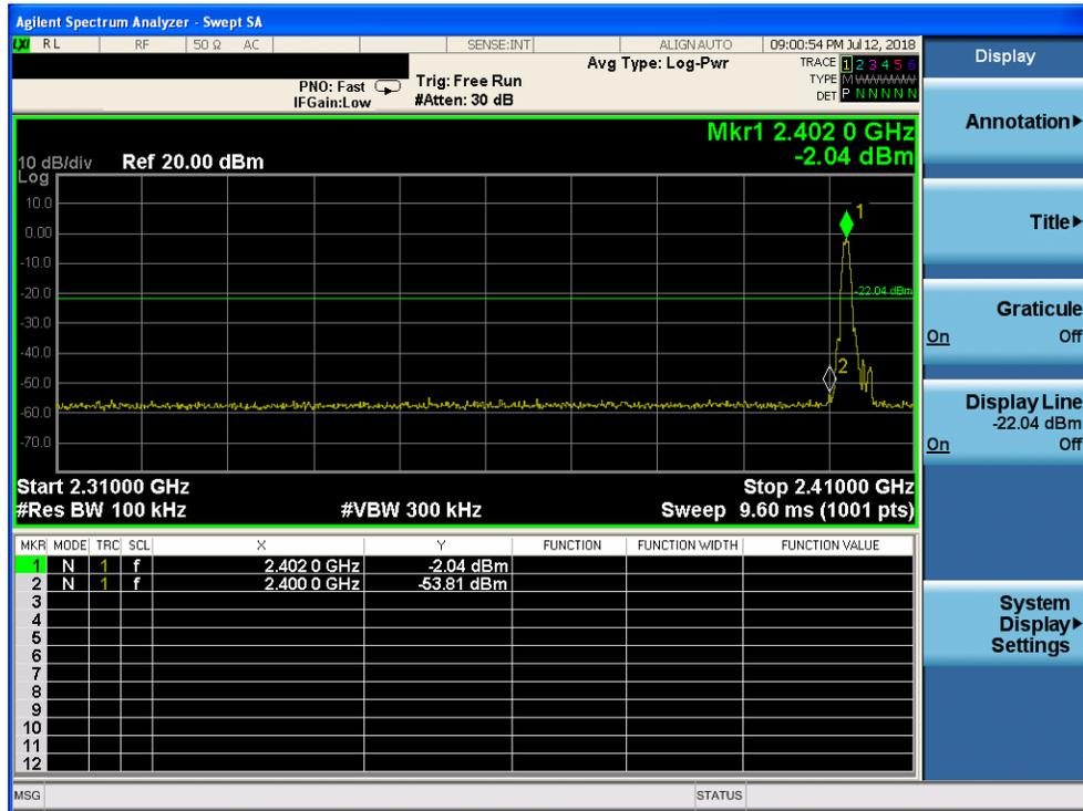
GFSK mode: Band Edge-High Channel
