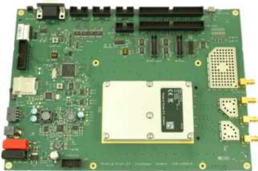
Figure 3-5: BGAN XL Radio Module carrier board
