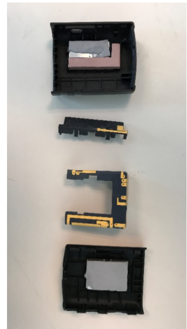
EUT Antenna and cover
