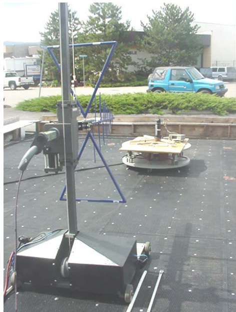
Photograph B.7-7 - Dipole Substitution Setup
