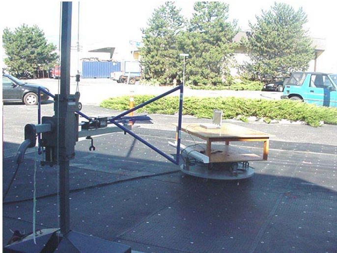
Photograph B.7-3 - Dipole Substitution Setup
