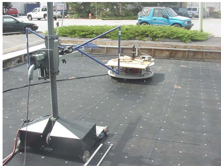
Photograph B.7-3 - Dipole Substitution Setup
