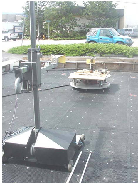
Photograph B.7-8 - Horn Substitution Setup
