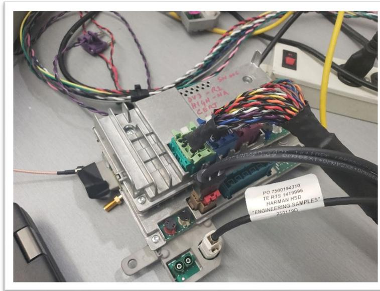
2.) Connect the white display cable from head unit as well as black display power cable to the display.
