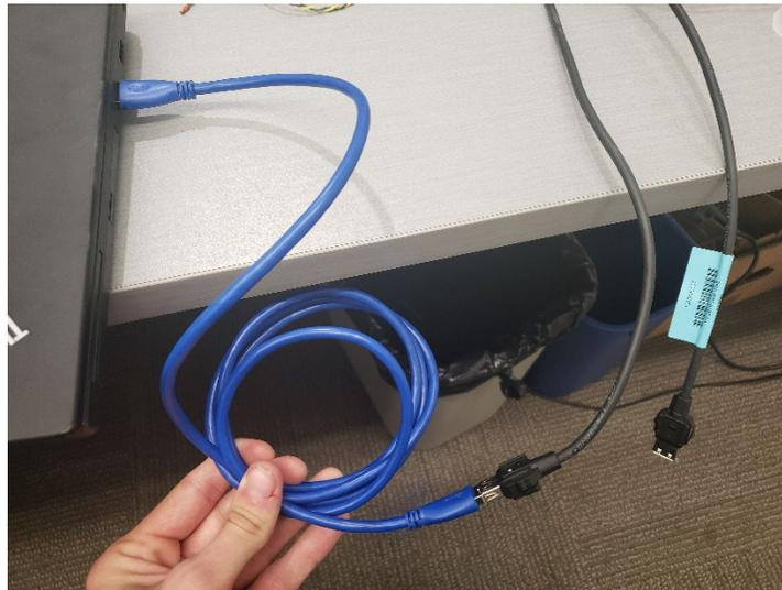
7.) Connect a USB to ethernet adapter to the brown and red USB cable. Then connect an ethernet cable from the USB to ethernet adapter to your PC as shown below.
