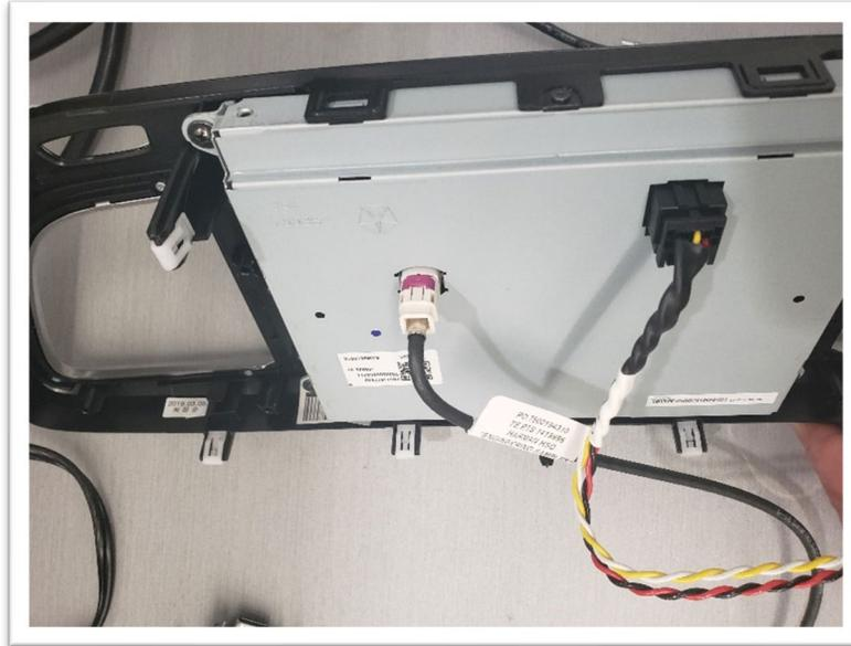
3.) On the Main Wiring Harness, identify the CAN IHS and CAN BH connectors.
