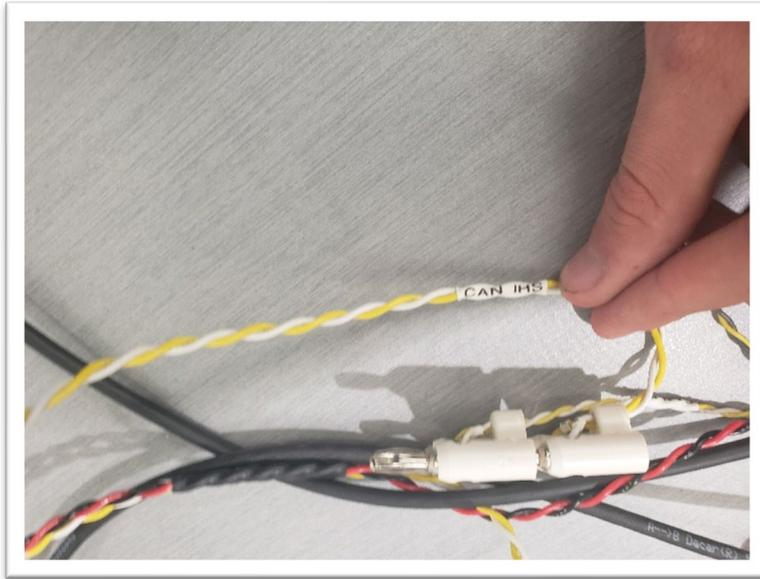
4.) Connect these 2 connectors and make sure white cables align with white cables and yellow with yellow as shown below.
