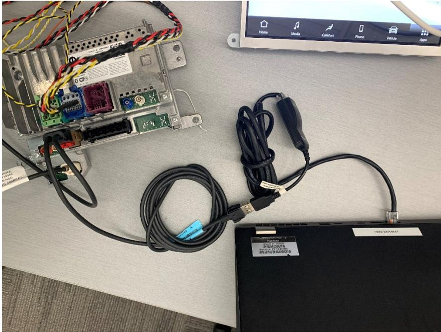
8.) Turn on Power Supply. Radio will boot in about 20 seconds.
