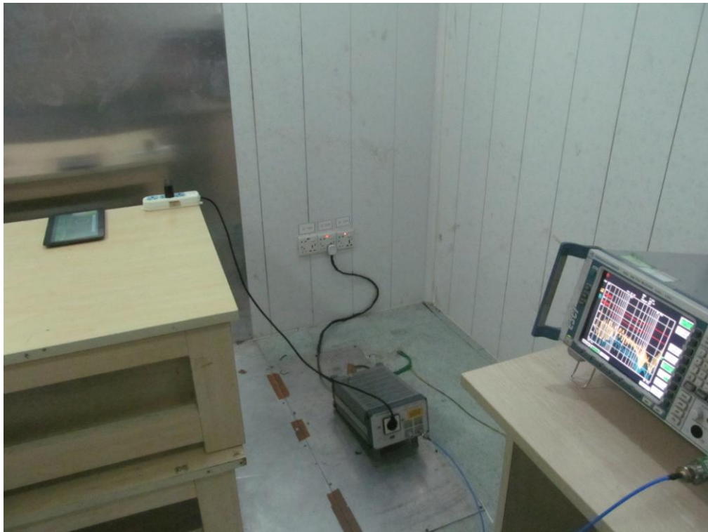
FCC RADIATED EMISSION TEST SETUP
