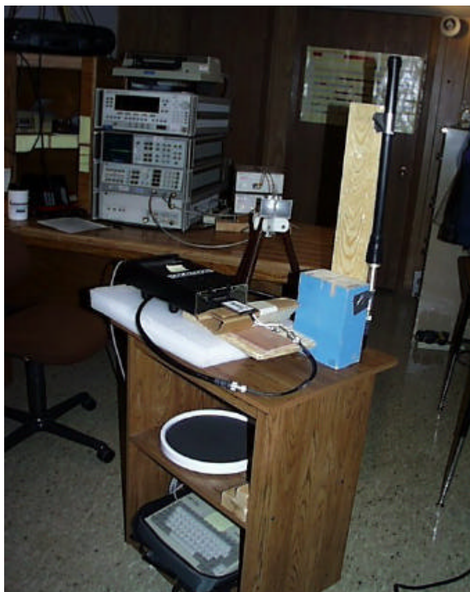
Photo 12: Shows placement of the 2126 radio with Mobile Mark antenna >18 GHz testing.
