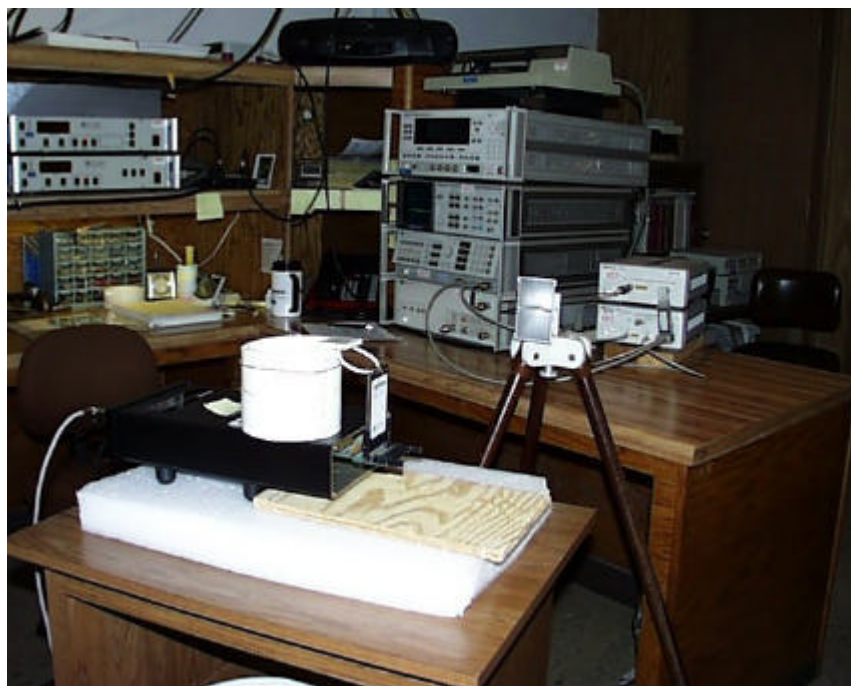
Photo 11: Shows vertical placement of the 2126 radio with Radiall antenna >18 GHz testing.
