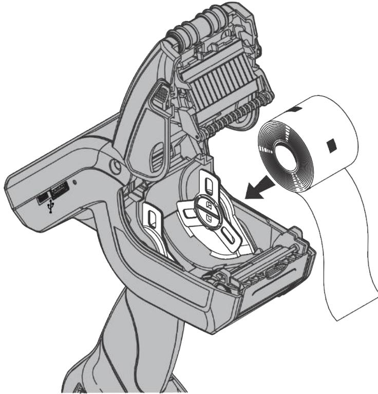
6. Continue loading supply for the printing mode you need: [peel](#) or [non-peel](#).
