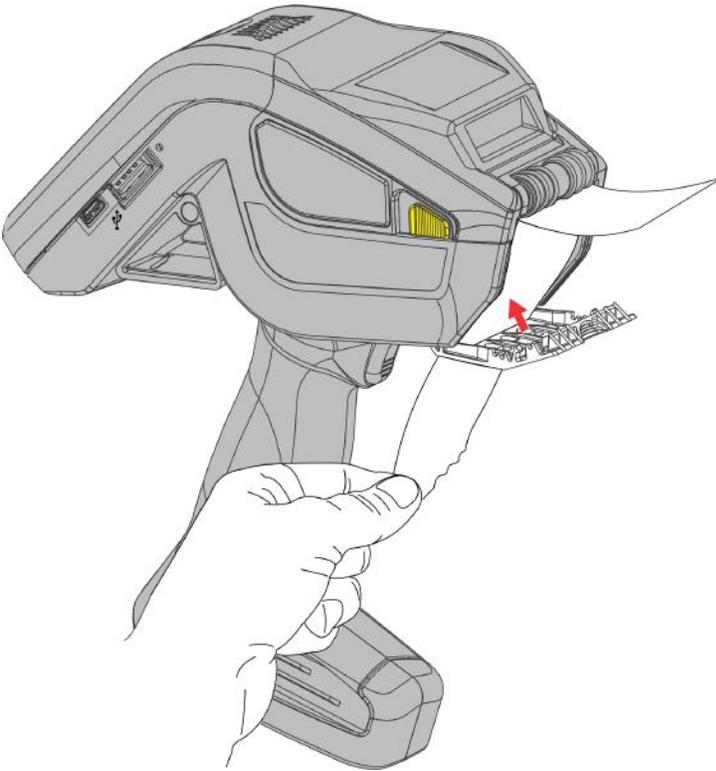
5. Hold the backing paper and push up the label deflector until it snaps into place.
