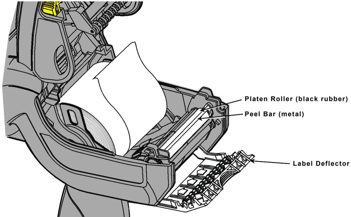
3. Feed the backing paper **over** the peel bar and through the slot at the base of the label deflector.
