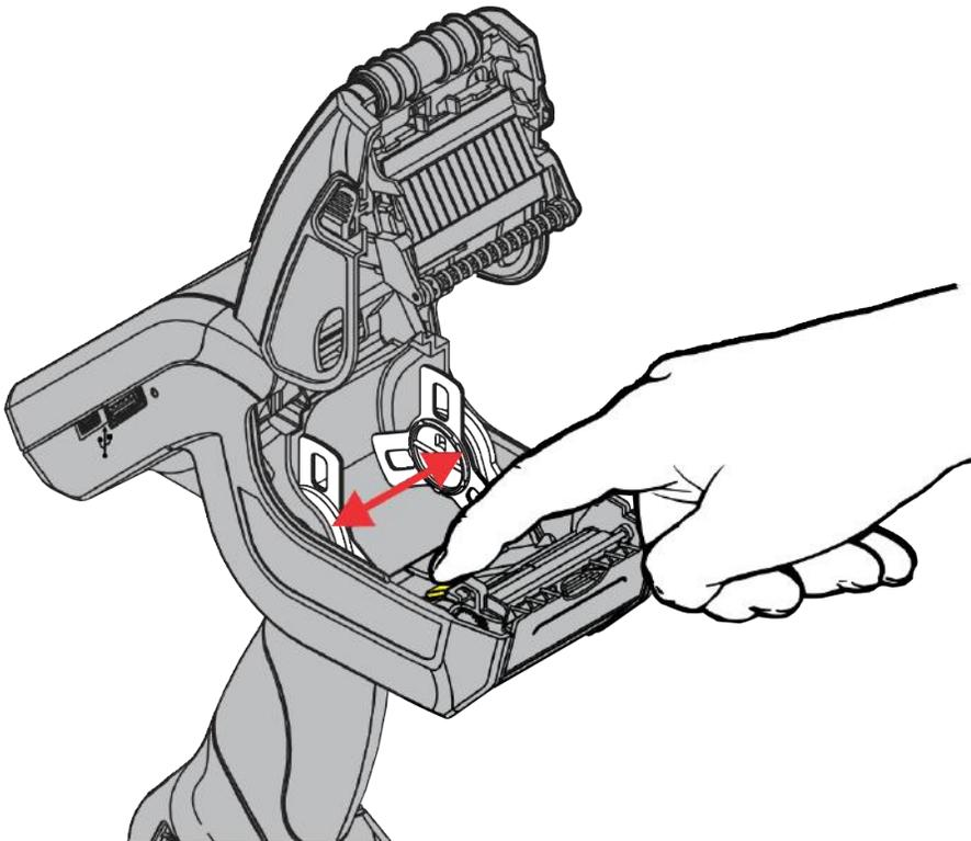
5. Place the supply roll in the supply holder so the supply unrolls from the bottom.
