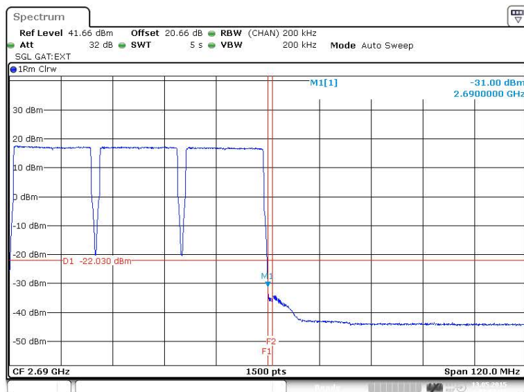
Figure 360 Spurious Emissions (Lower Band Edge) – 64QAM (2506/2526.0/2546.0 MHz) (20MHz Channel BW)
