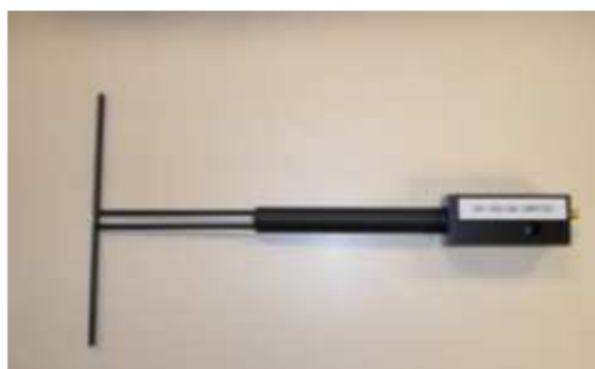
Figure 1 – Satimo COMOSAR Validation Dipole
