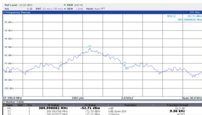
Figure 8.4-15: 20 dB bandwidth, Genie, Intellicode® II, 2010-2011, 390 MHz
