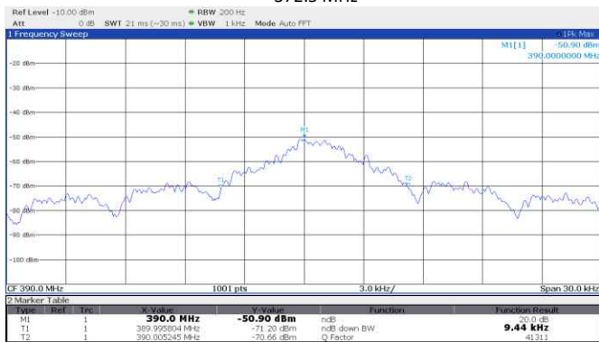
Figure 8.4-11: 20 dB bandwidth, Genie, Intellicode® I, 1995-current, 390 MHz
