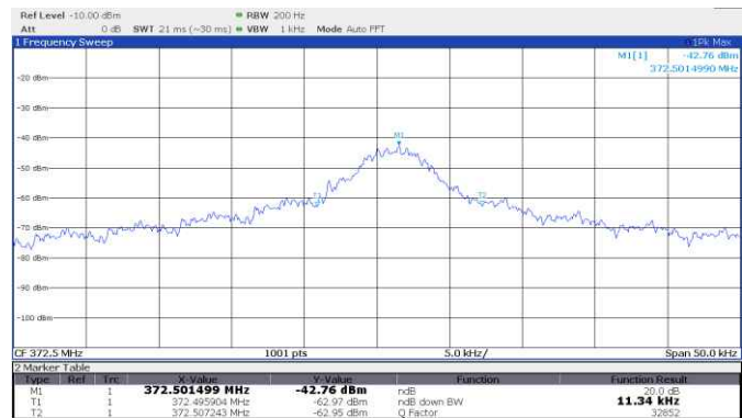
Figure 8.4-10: 20 dB bandwidth, Ryobi, rolling code, 372.5 MHz
