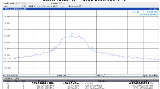
Figure 8.5-14: 99% occupied bandwidth, Chamberlain, Green learn button, Billion Code®, 1993-1995, 390 MHz
