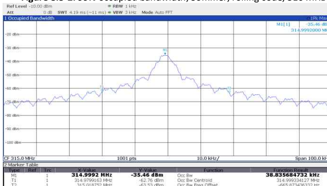
Figure 8.5-4: 99% occupied bandwidth, Genie, Intellicode®, 1995-current, 315 MHz
