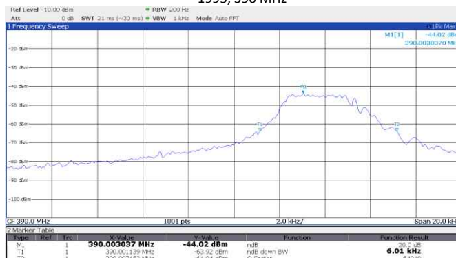
Figure 8.4-19: 20 dB bandwidth, OHD, 9 switch/3 position DIP switch, 1993-1995, 390 MHz
