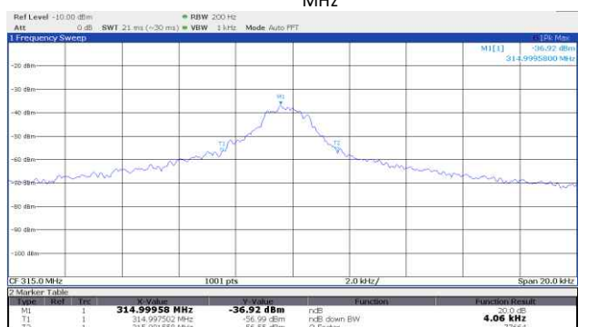
Figure 8.4-5: 20 dB bandwidth, Chamberlain, purple learn button, security+, 2006-2014, 315 MHz
