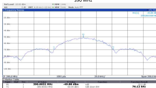
Figure 8.4-18: 20 dB bandwidth, Genie, 9 switch/2 position DIP switch, 1993-1995, 390 MHz
