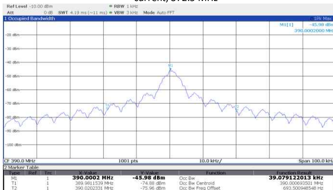
Figure 8.5-11: 99% occupied bandwidth, Genie, Intellicode® I, 1995-current, 390 MHz
