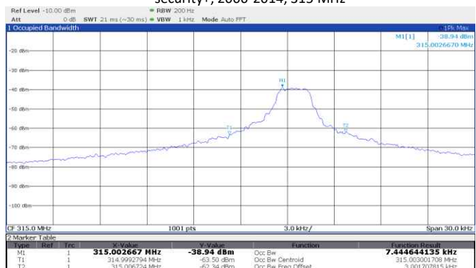
Figure 8.5-7: 99% occupied bandwidth, Marantec, fixed learn code, 315 MHz
