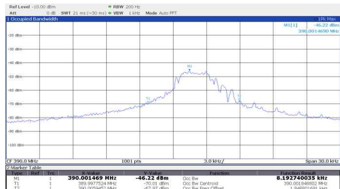
Figure 8.5-12: 99% occupied bandwidth, Chamberlain, Orange/Red learn button, Security+®, 1996-2005, 390 MHz
