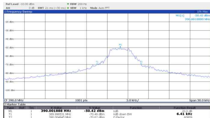
Figure 8.4-12: 20 dB bandwidth, Chamberlain, Orange/Red learn button, Security+®, 1996-2005, 390 MHz
