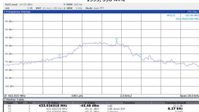
Figure 8.4-20: 20 dB bandwidth, FAAC, Rolling code, 433.92 MHz
