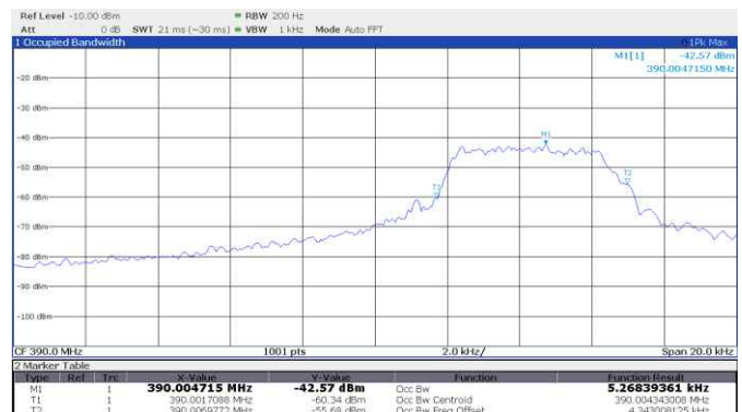
Figure 8.5-16: 99% occupied bandwidth, Chamberlain, 9 switch / 3 position DIP switch, 390 MHz
