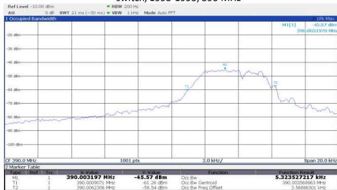
Figure 8.5-19: 99% occupied bandwidth, OHD, 9 switch/3 position DIP switch, 1993-1995, 390 MHz
