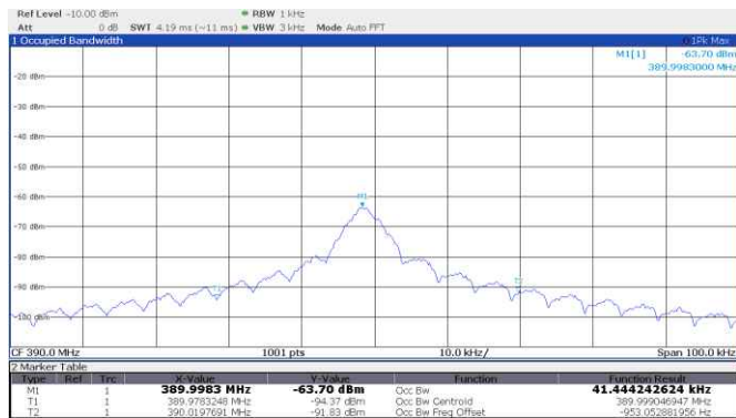
Figure 8.5-15: 99% occupied bandwidth, Genie, Intellicode® II, 2010-2011, 390 MHz
