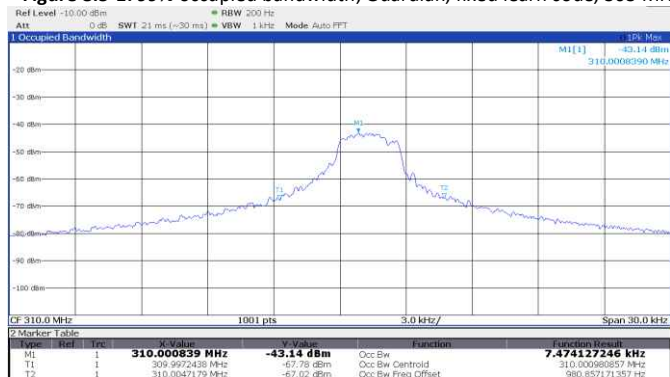
Figure 8.5-3: 99% occupied bandwidth, Stanley, 10 switch / 2 position DIP switch, 310 MHz
