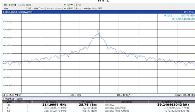
Figure 8.5-6: 99% occupied bandwidth, Genie, Intellicode® II, 2010-2010, 315 MHz
