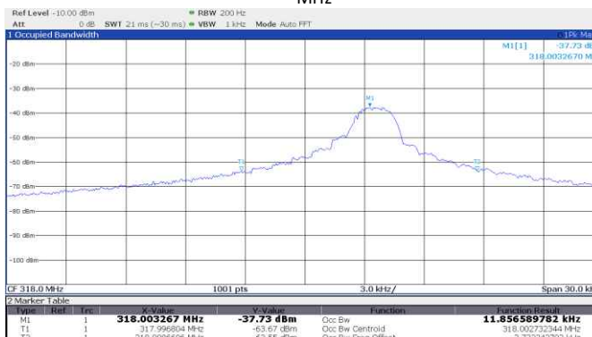
Figure 8.5-8: 99% occupied bandwidth, Linear, Mega Code®, 318 MHz
