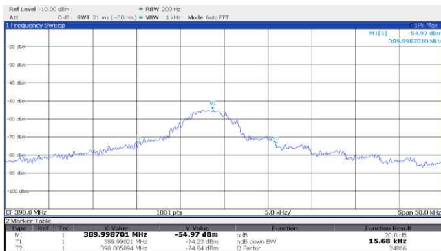
Figure 8.4-13: 20 dB bandwidth, Chamberlain, Yellow learn button, Security+2.0®, 2011-current, 390 MHz
