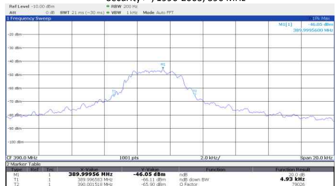
Figure 8.4-14: 20 dB bandwidth, Chamberlain, Green learn button, Billion Code®, 1993-1995, 390 MHz
