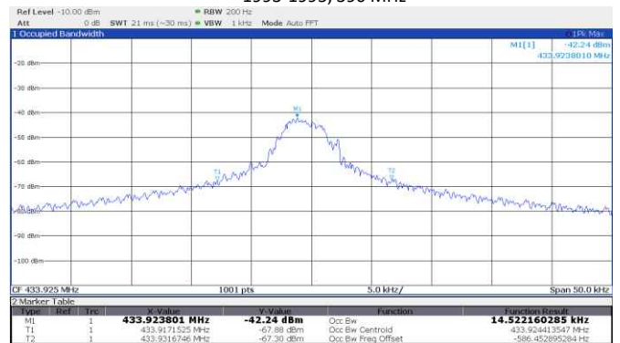
Figure 8.5-20: 99% occupied bandwidth, FAAC, Rolling code, 433.92 MHz
