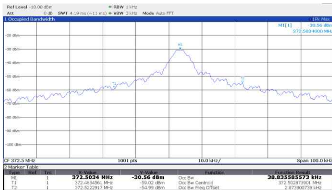
Figure 8.5-9: 99% occupied bandwidth, Wayne Dalton, rolling code, 1999-current, 372.5 MHz
