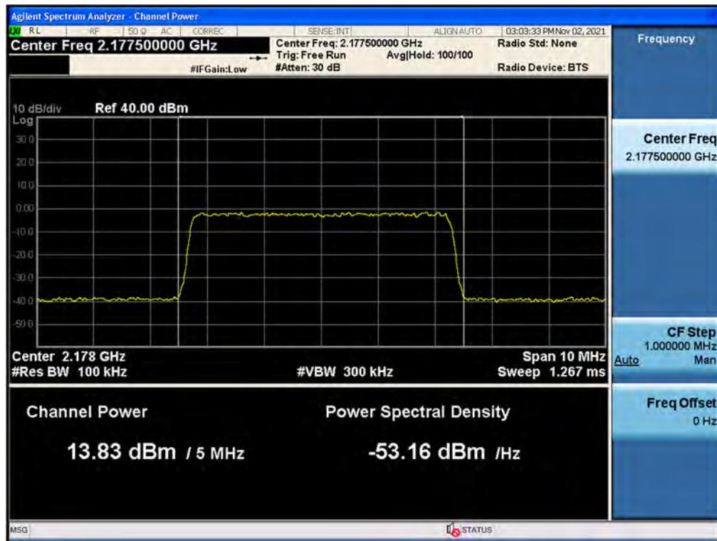
**Antenna 1 / B66 LTE 20 MHz 1 Carrier + B66 LTE 10 MHz 1 Carrier [2 Carrier] / Non-Contiguous / B66 LTE 20 MHz / QPSK / Low**
