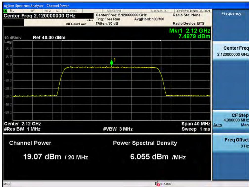
**Antenna 1 / 5G NR n66 20 MHz 1 Carrier + 5G NR n66 10 MHz 1 Carrier [2 Carrier] / Non-Contiguous / 5G NR n66 10 MHz / 256QAM / High**
