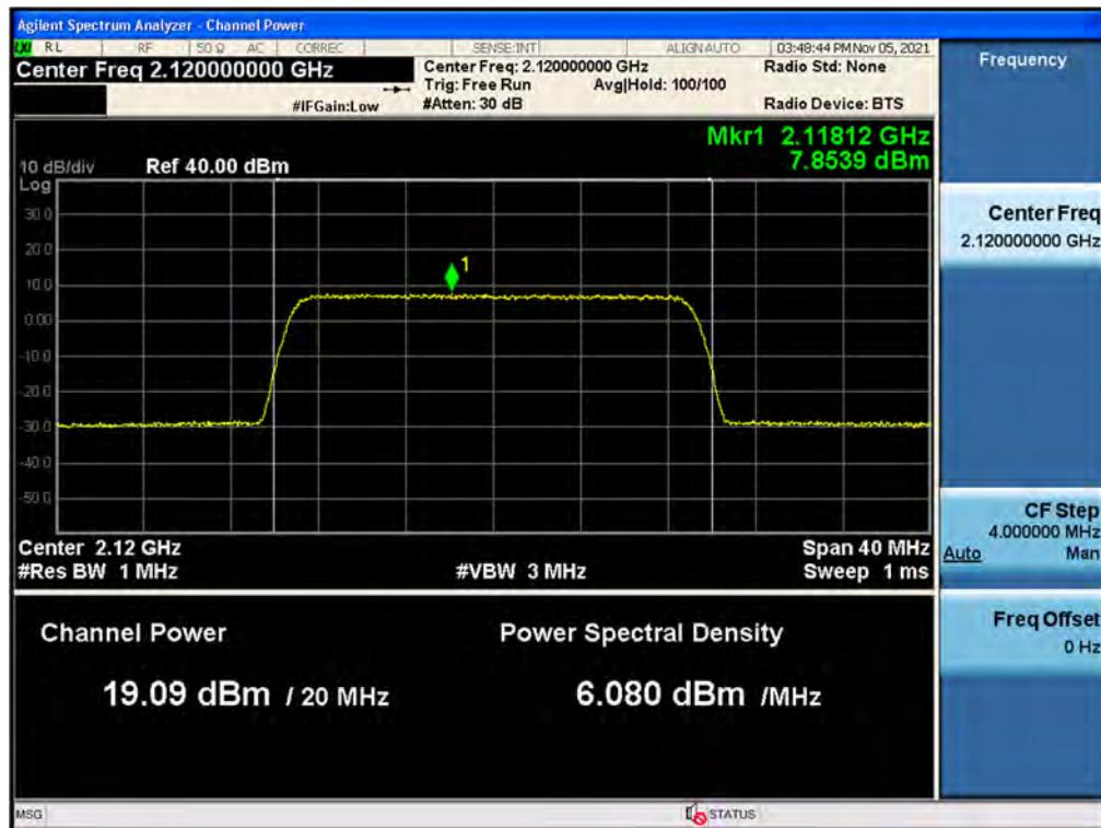
**Antenna 1 / B66 LTE 20 MHz 1 Carrier + 5G NR n66 10 MHz 1 Carrier [2 Carrier] / Non-Contiguous / 5G NR n66 10 MHz / QPSK / High**
