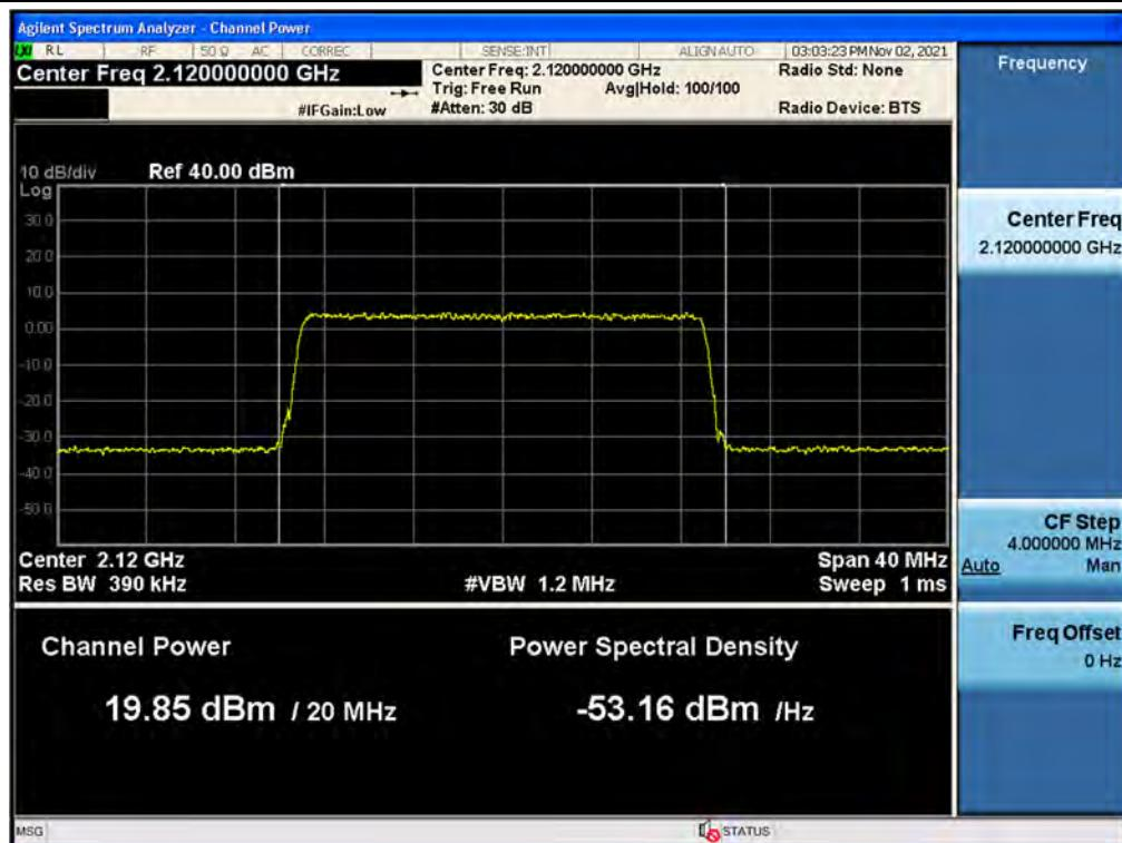
**Antenna 1 / B66 LTE 20 MHz 1 Carrier + B66 LTE 5 MHz 1 Carrier [2 Carrier] / Non-Contiguous / B66 LTE 5 MHz / QPSK / High**
