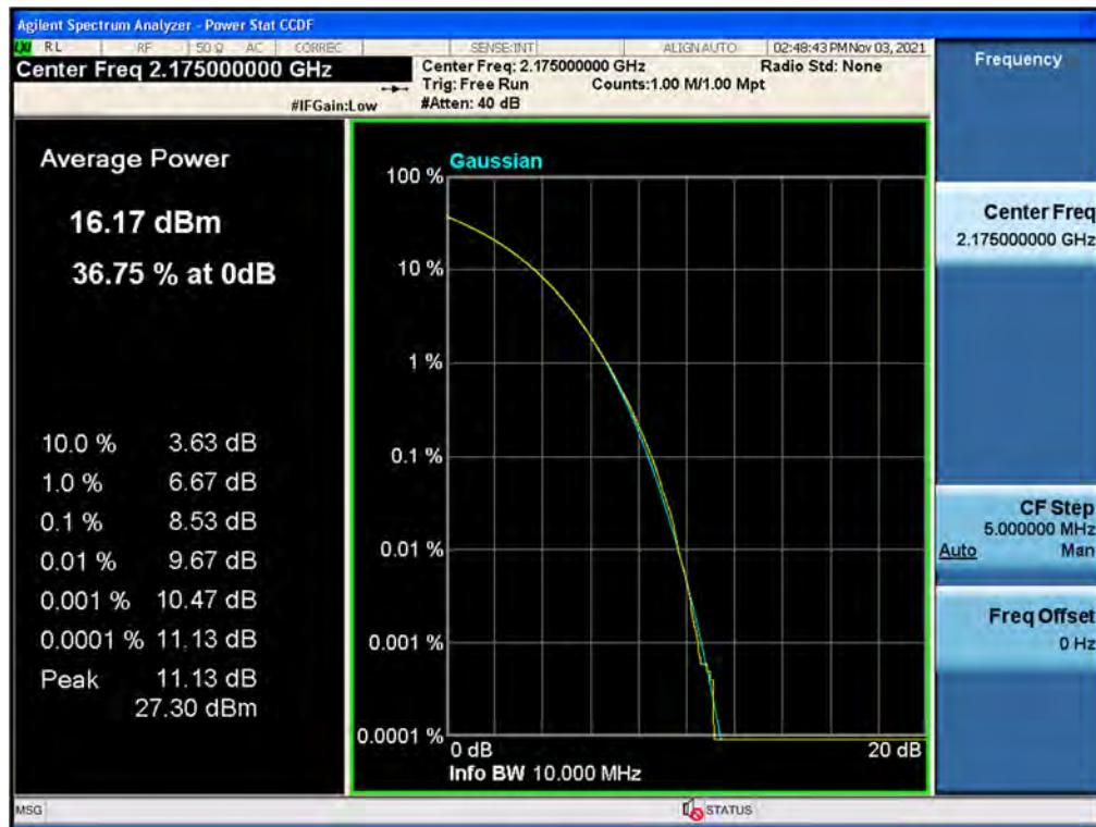
**Antenna 1 / 5G NR n66 5 MHz 1 Carrier + B66 LTE 5 MHz 1 Carrier [2 Carrier] / Non-Contiguous / 5G NR n66 5 MHz / 16QAM / Low**
