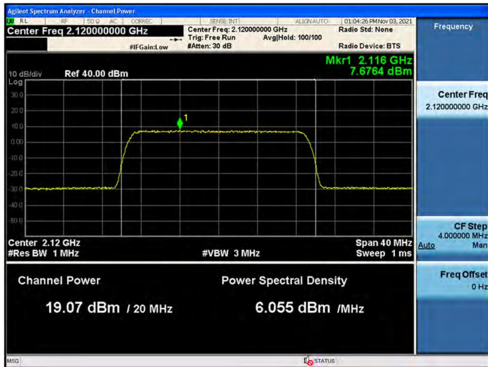
**Antenna 1 / B66 LTE 20 MHz 1 Carrier + B66 LTE 10 MHz 1 Carrier [2 Carrier] / Non-Contiguous / B66 LTE 10 MHz / QPSK / High**
