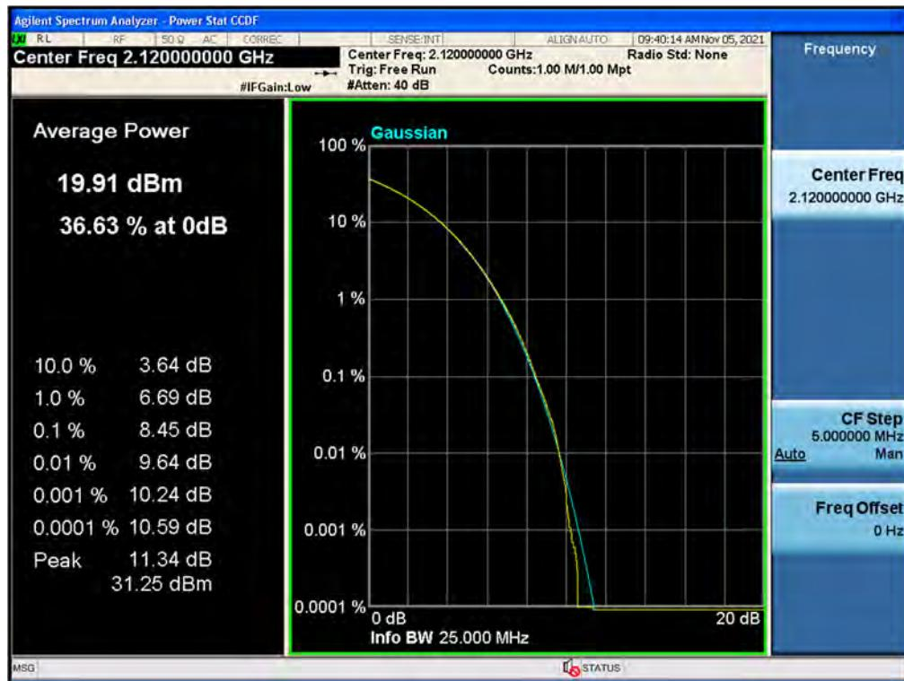
**Antenna 1 / 5G NR n66 20 MHz 1 Carrier + B66 LTE 5 MHz 1 Carrier [2 Carrier] / Non-Contiguous / B66 LTE 5 MHz / 256QAM / High**
