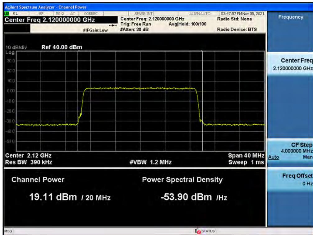
**Antenna 1 / B66 LTE 20 MHz 1 Carrier + 5G NR n66 10 MHz 1 Carrier [2 Carrier] / Non-Contiguous / 5G NR n66 10 MHz / QPSK / High**
