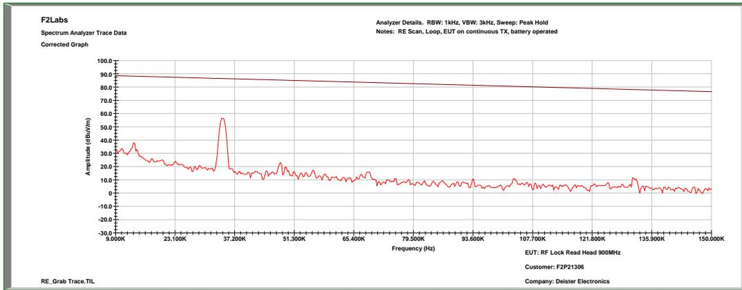
**900 MHz: 0.15 MHz to 30 MHz (Loop Antenna)**
