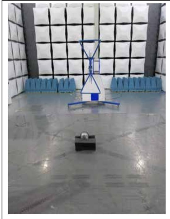
900 MHz: Radiated Spurious Emissions (Loop Antenna)
