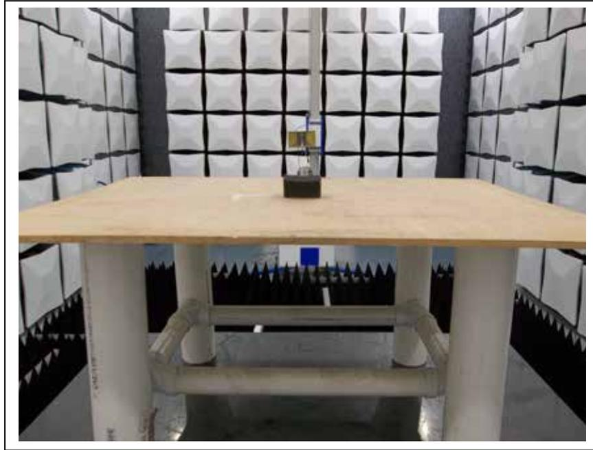
**2.4 GHz: Radiated Spurious Emissions (Loop Antenna)**
