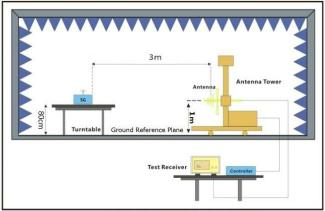
Substitue Antenna+Signal Generator
