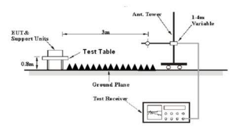
The radiated emission tests were performed in the 3 meters chamber test site, using the setup accordance with the ANSI C63.4-2014. The specification used was the FCC Part 15.109 Class B limits.
