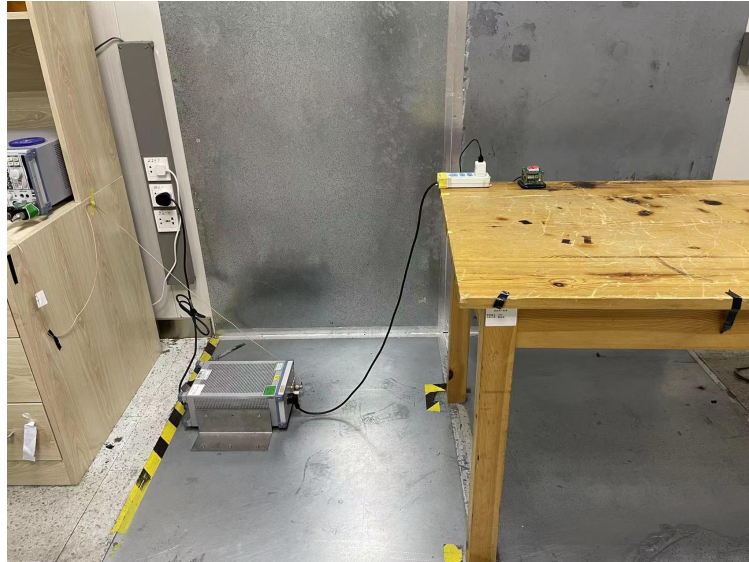
Radiated Spurious Emissions Test Frequency From 9KHz-30MHz
