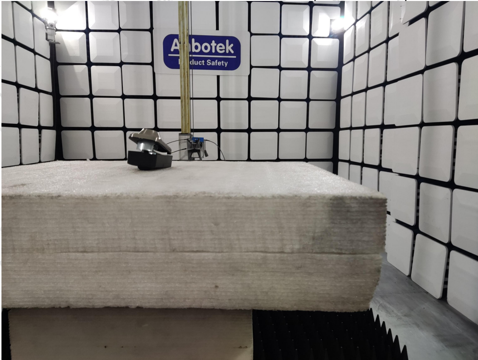
Photo of Radiation Emission Test (above 1GHz)
