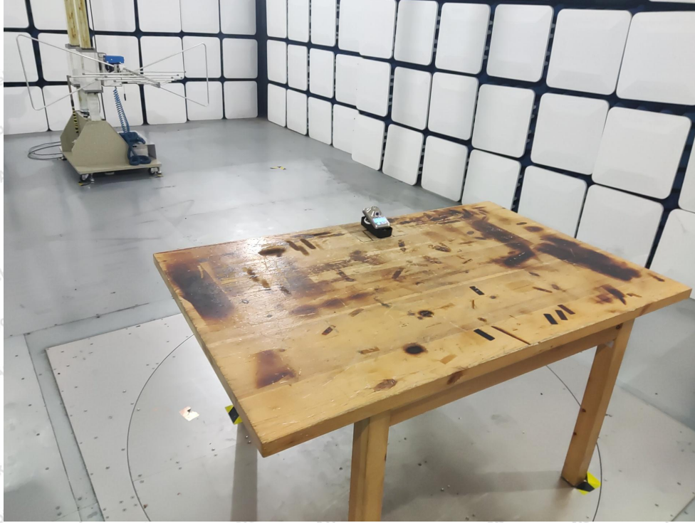
Photo of Radiation Emission Test (below 1GHz)
