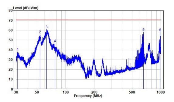
Site : chamber Condition: 3m VERTICAL Job No. : SZ2220426-16719E-EMA1 Test Mode: Microwave
