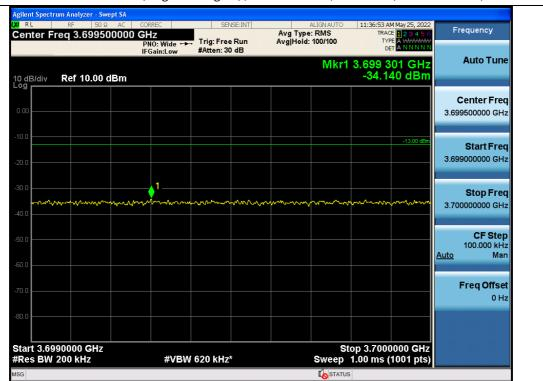
+3 dB above Out-of-band (single test signal) / C-Band ANT 2 / Downlink / 5G NR 20 MHz / Lower
