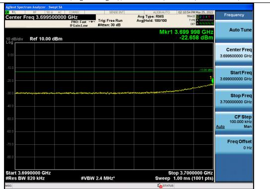
+3 dB above Out-of-band (single test signal) / C-Band ANT 2 / Downlink / 5G NR 80 MHz / Lower
