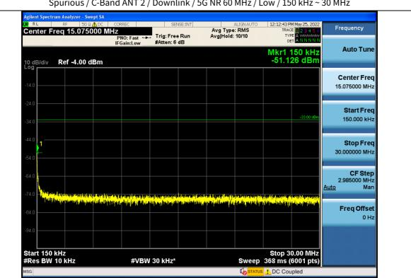
Spurious / C-Band ANT 2 / Downlink / 5G NR 60 MHz / Low / 150 kHz ~ 30 MHz
