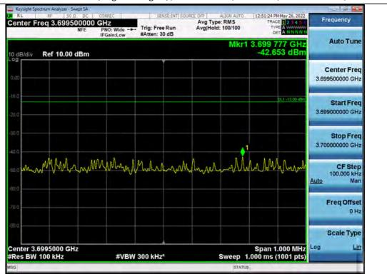
+3 dB above Out-of-band (single test signal) / C-Band ANT 2 / Downlink / 5G NR 100 MHz / Lower
