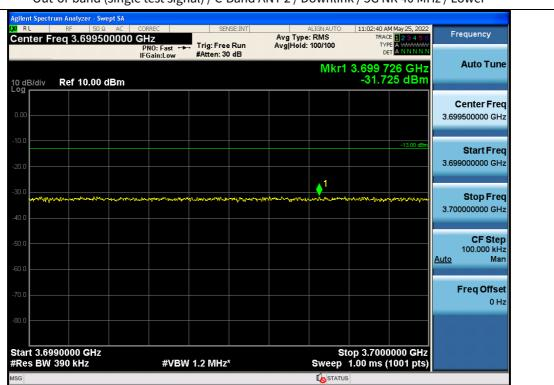
Out-of-band (single test signal) / C-Band ANT 2 / Downlink / 5G NR 40 MHz / Lower
