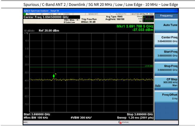
Note: Limit compensation:  $-13 \text{ dBm} - 10 \log(2) - 10 \text{ dB} = -26.01 \text{ dBm}$
