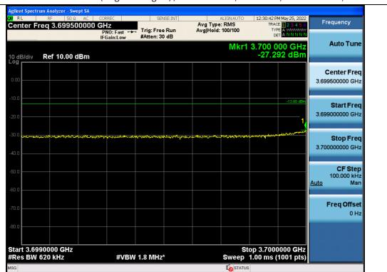
+3 dB above Out-of-band (single test signal) / C-Band ANT 2 / Downlink / 5G NR 60 MHz / Lower
