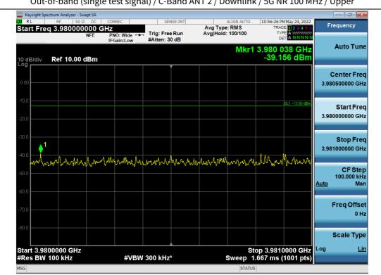
Out-of-band (single test signal) / C-Band ANT 2 / Downlink / 5G NR 100 MHz / Upper
