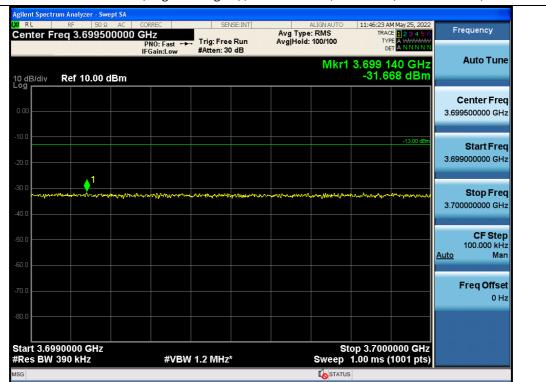
+3 dB above Out-of-band (single test signal) / C-Band ANT 2 / Downlink / 5G NR 40 MHz / Lower
