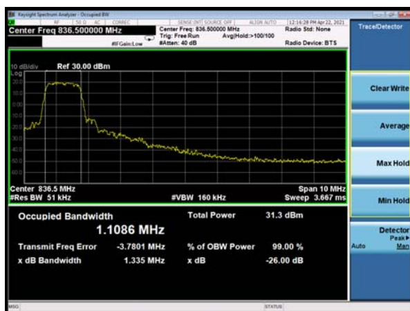
LTE Band 5 QPSK 10MHz CH-Middle
