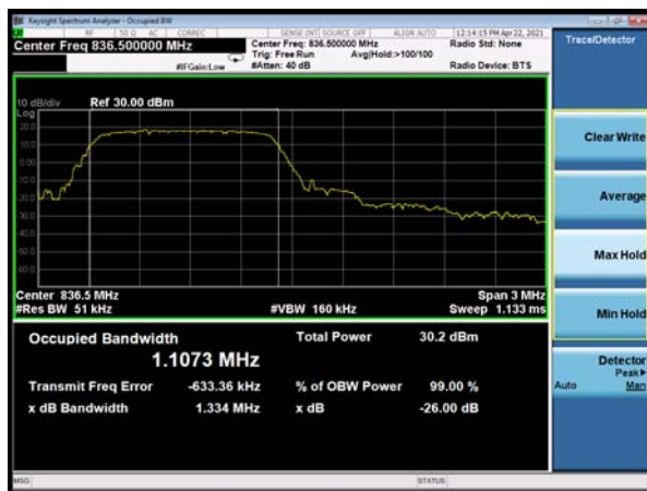
LTE Band 5 QPSK 10MHz CH-Middle
