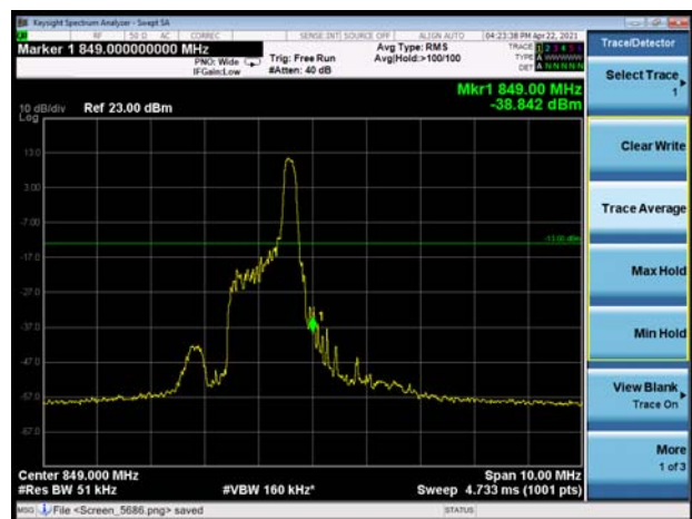
LTE Band 5 16QAM 3MHz CH-High 100%RB
