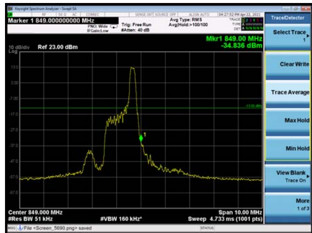
LTE Band 5 16QAM 5MHz CH-High 100%RB
