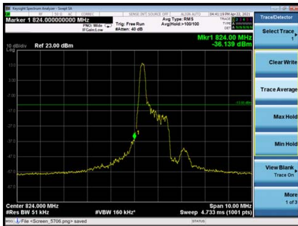
LTE Band 5 16QAM 5MHz CH-Low 100%RB
