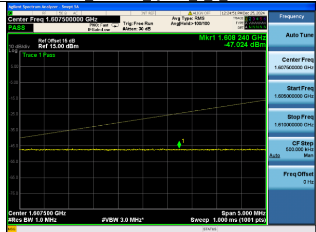
Band255 3.75kHz QPSK 1 0 CH261672
