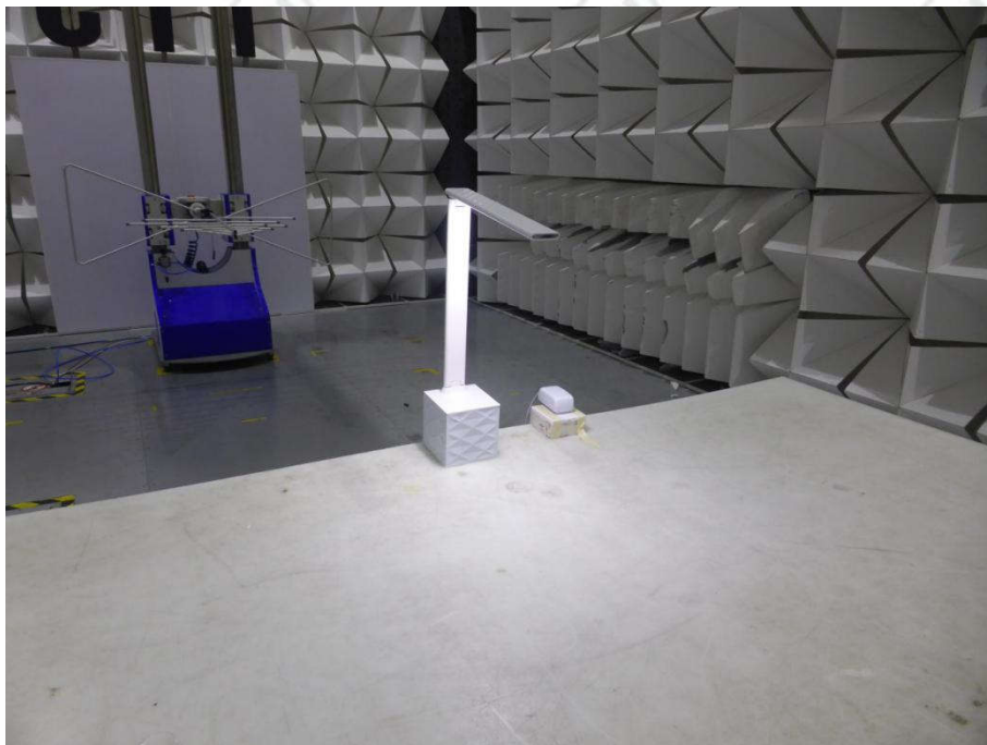
Radiated spurious emission Test Setup-1(Below 1GHz)
