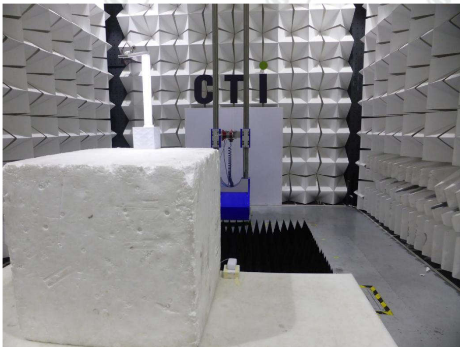
Radiated spurious emission Test Setup-2(Above 1GHz)
