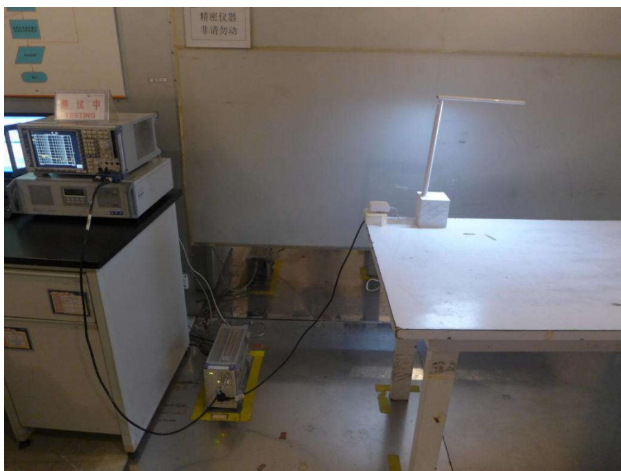
Conducted Emissions Test Setup
