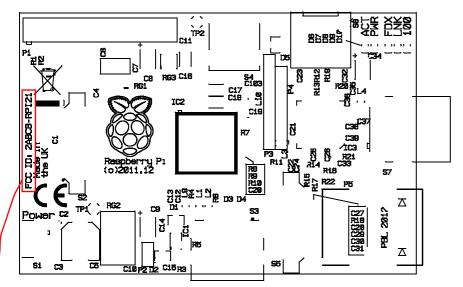
This is the position of the FCC ID. The diagram is taken from the design file, hence the image quality is low. The FCC ID will be reproduced exactly as follows:
