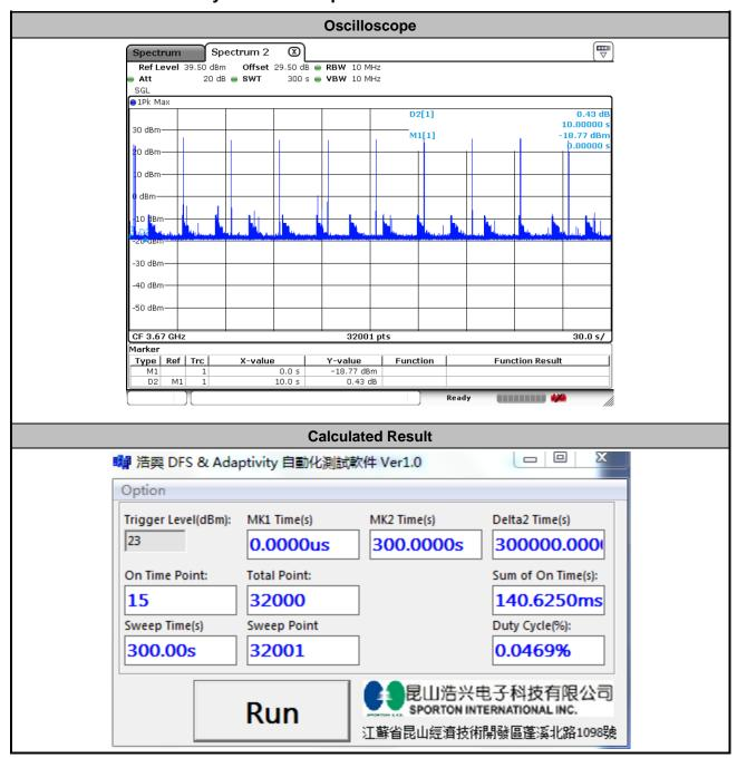
The sum of On Time (aggregated time from marker 1 to 2): 140.625ms < 10s, Pass.
