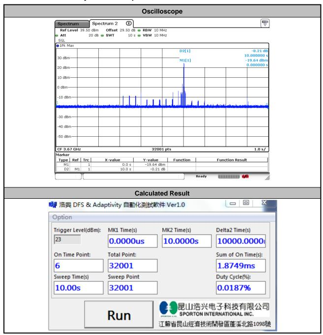
The sum of On Time (aggregated time from marker 1 to 2): 1.8749ms < 1s, Pass.
