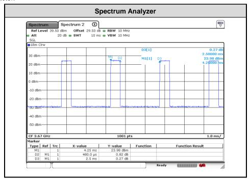
Note: The duty cycle value is 19.20%, add 10log(1/duty cycle) to the measured power level to compute the average power during continuous transmission.
