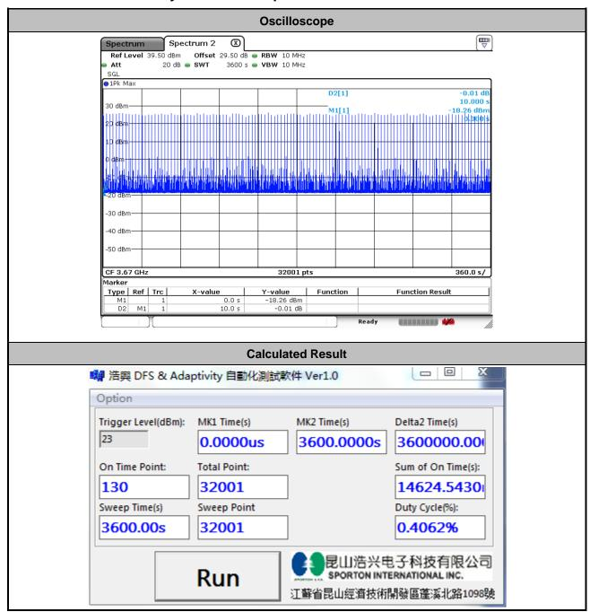
The sum of On Time (aggregated time from marker 1 to 2): 14624.543ms < 20s, Pass.
