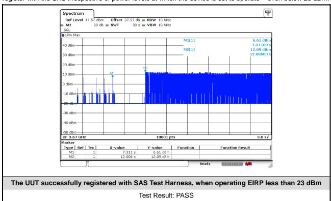
Note: The Ref Offset 37.57 dB includes the antenna gain13.00 dBi and cable path loss 24.57dB.
