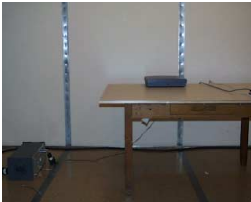
Photo 5 – Conducted Emissions Test Setup – Front View
