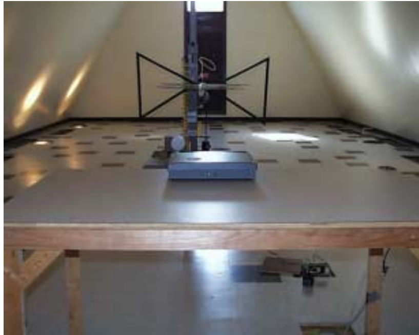
Photo 2 – Radiated Emissions Test Setup – Front View
