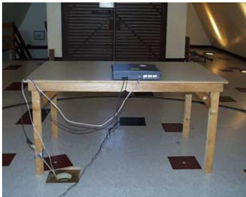
Photo 3 – Radiated Emissions Test Setup – Rear View
