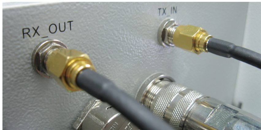
SMA Coaxial Cable Inter-connection on Single-band Enclosure
