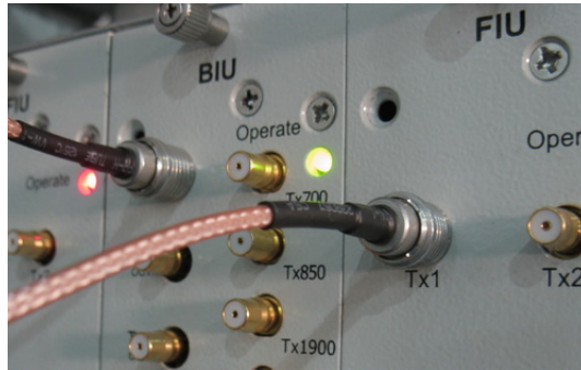
Figure 21 BTS QMA Coaxial Cable Connection
