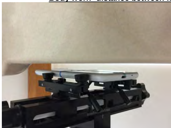
Fig.7 EUT Front side to flat phantom
