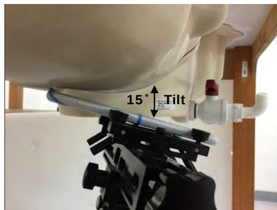
Fig.4 Right Head Section / Ear-Tilt Position(15°)
