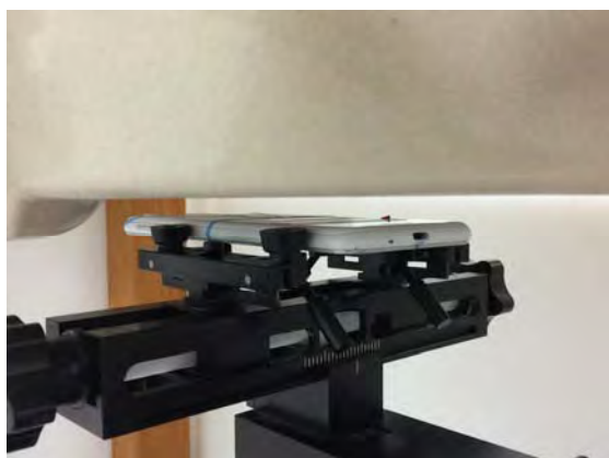
Fig.8 EUT Back side to flat phantom
