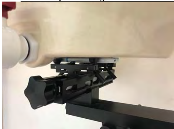
Fig.15 EUT Front side to flat phantom
