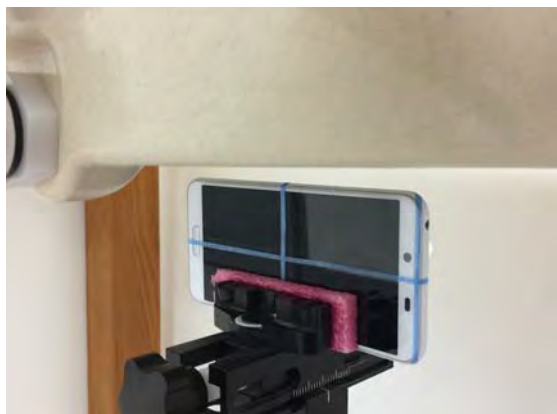
Fig.14 EUT Left side to flat phantom
