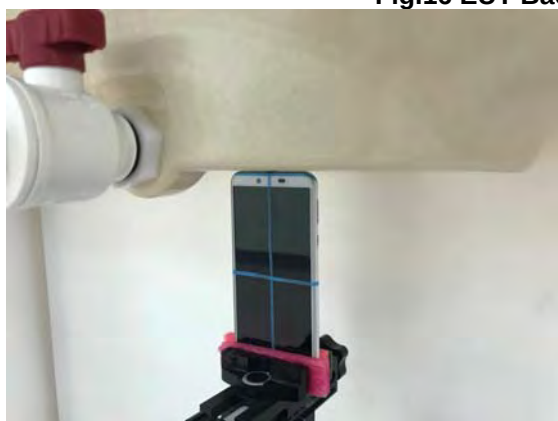
Fig.17 EUT Top side to flat phantom
