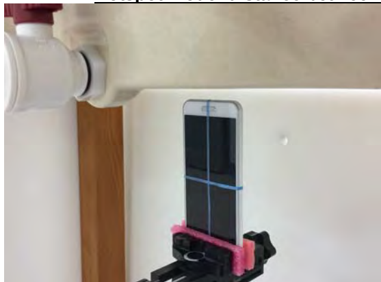
Fig.12 EUT Bottom side to flat phantom
