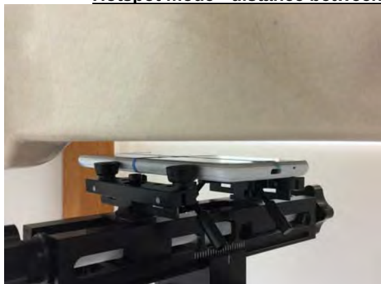
Fig.9 EUT Front side to flat phantom
