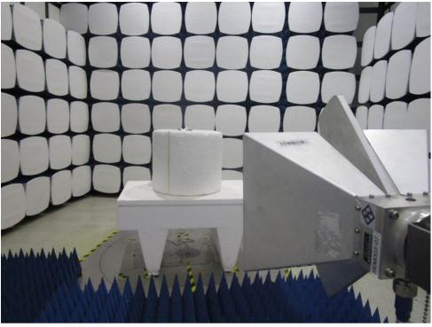
1.2 Radiated Spurious Emissions Test Setup
