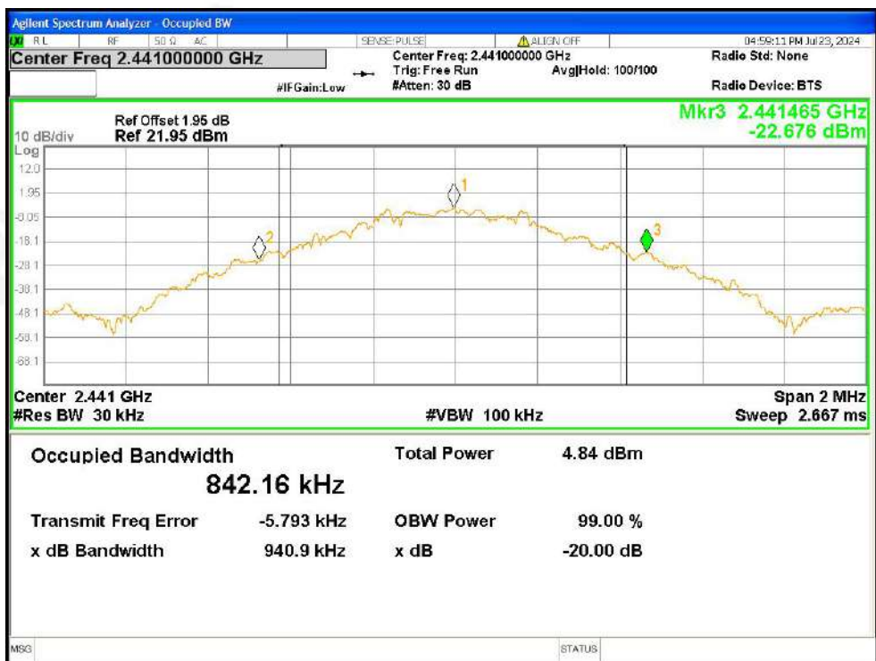
-20dB Bandwidth NVNT 1-DH5 2441MHz Ant1
