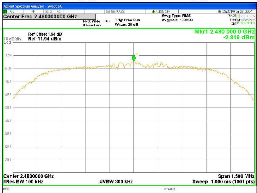
Tx. Spurious NVNT 3-DH5 2480MHz Ant1 Ref
