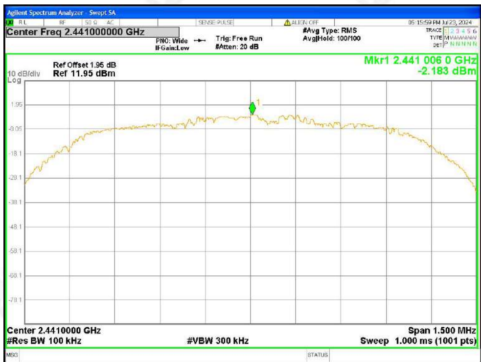
Tx. Spurious NVNT 3-DH5 2441MHz Ant1 Ref
