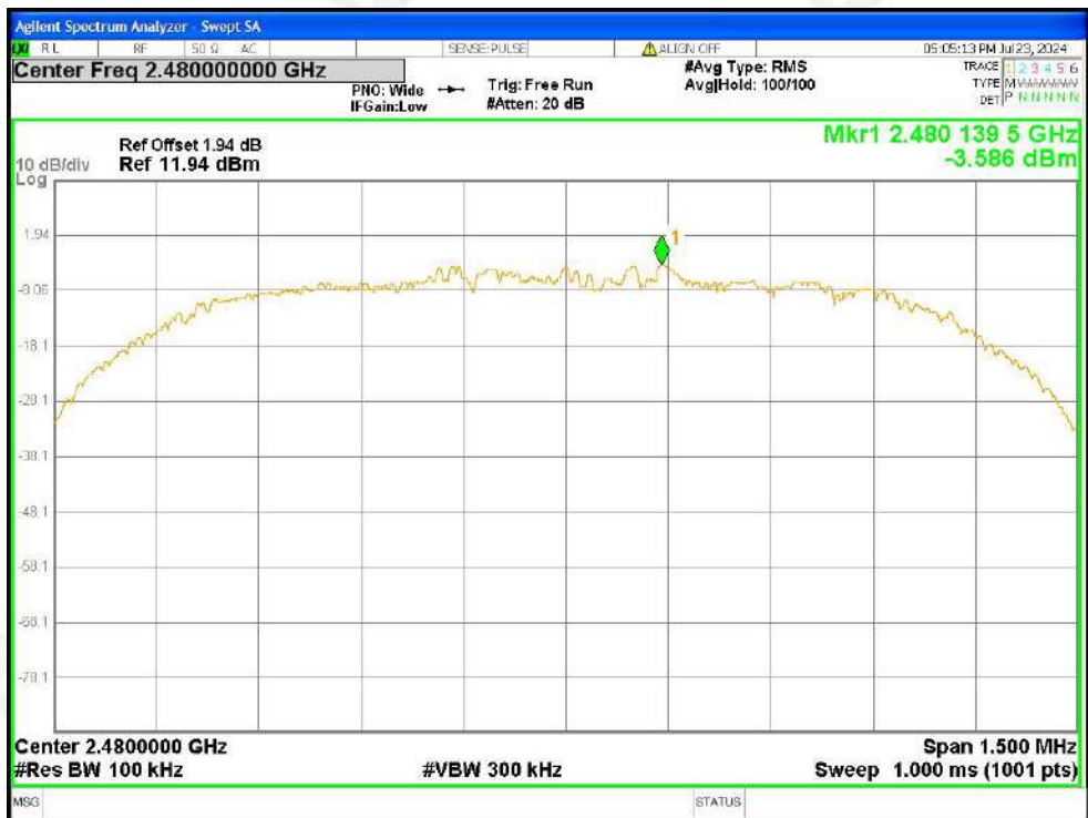
Tx. Spurious NVNT 2-DH5 2480MHz Ant1 Ref
