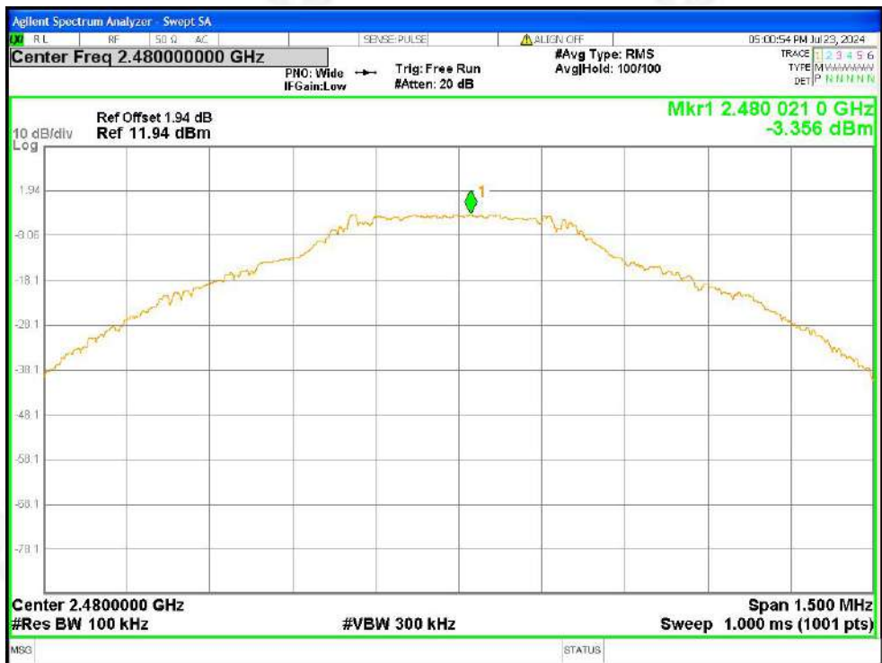
Tx. Spurious NVNT 1-DH5 2480MHz Ant1 Ref
