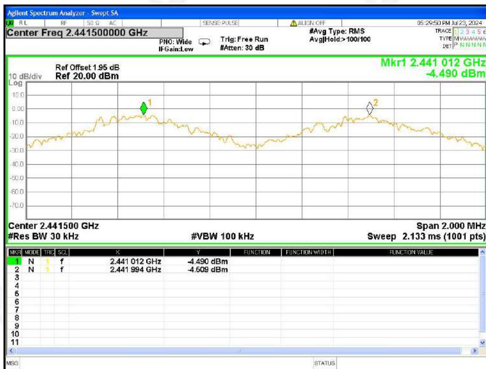
CFS NVNT 1-DH5 2441MHz Ant1
