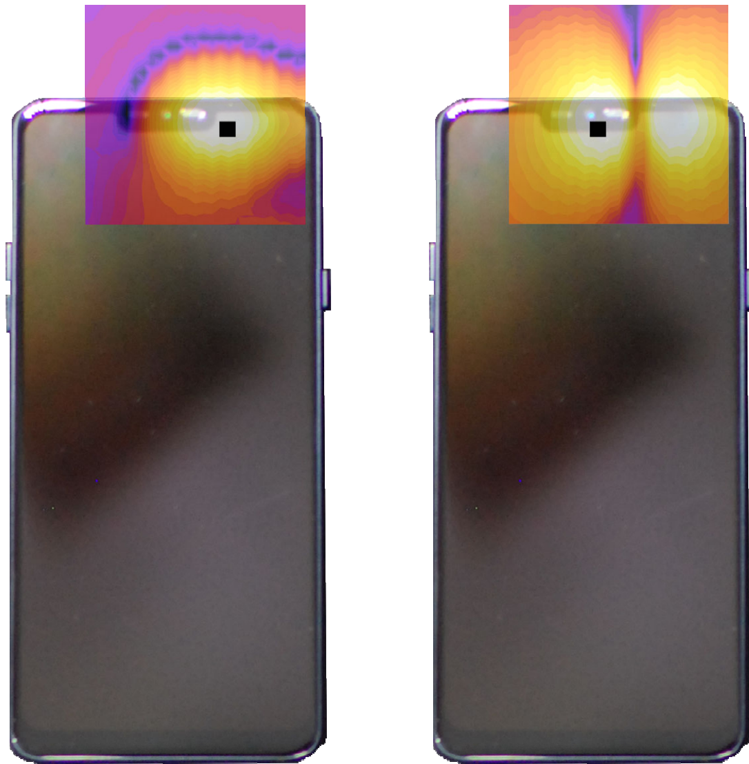
Figure 16-3 T-Coil Scan Overlay Magnetic Field Distributions
