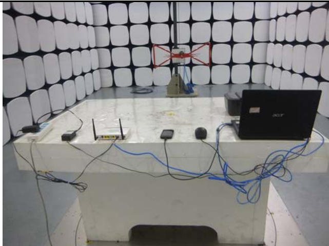
Radiated Emissions Test Setup Below 1GHz
