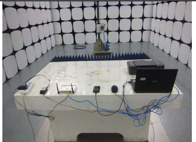
Radiated Emissions Test Setup Above 1GHz
