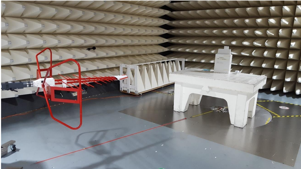
3. Radiated Emission test setup Low Range
