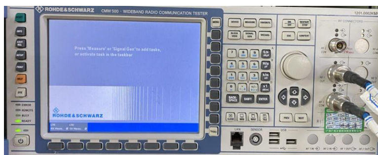
CMW 500 (2G/3G/4G Test Equipment)
