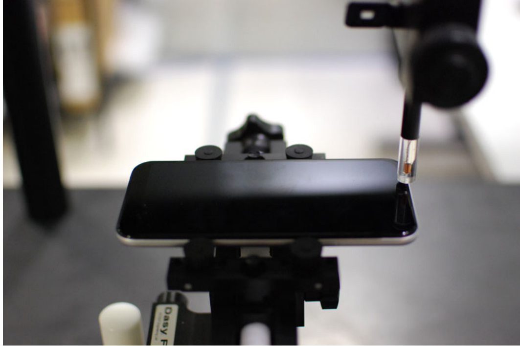
Figure 16-1 Test Setup for Wireless Device
