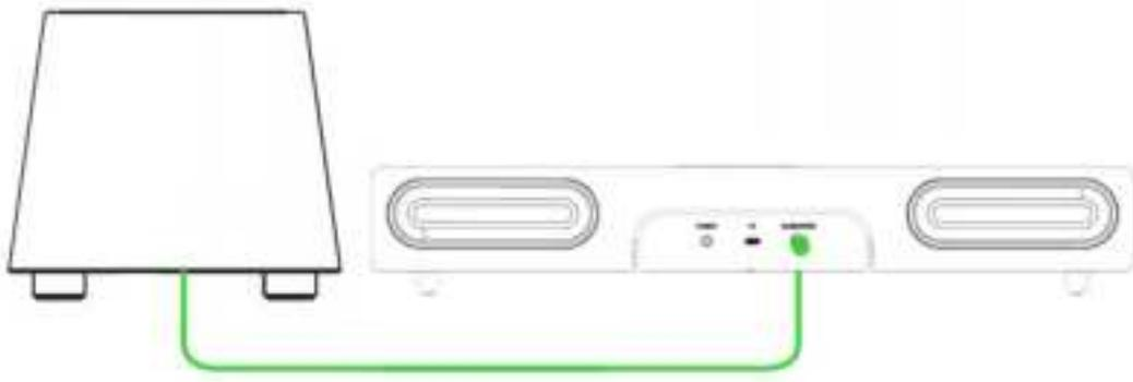
**i** *Make sure to press down on the connector catch clip before plugging/unplugging the subwoofer connector.*
