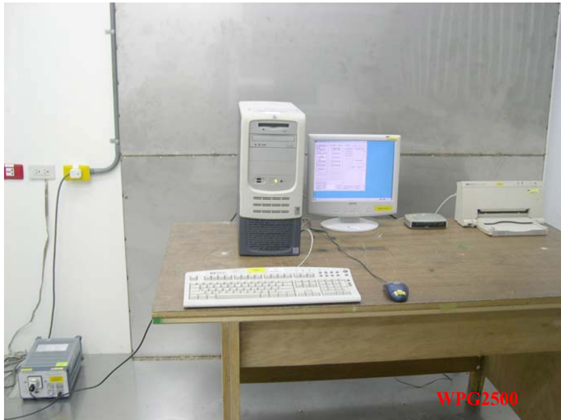
Photo 1: Conducted Emission Test Set-up
