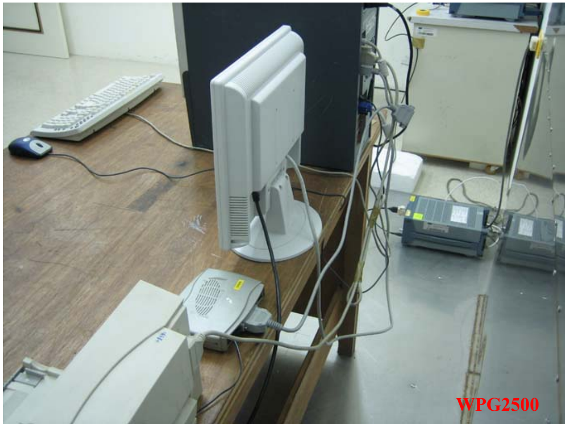
Photo 2: Conducted Emission Test Set-up
