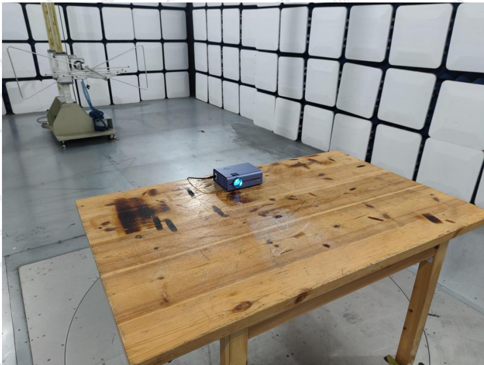
Photo of Radiation Emission Test
