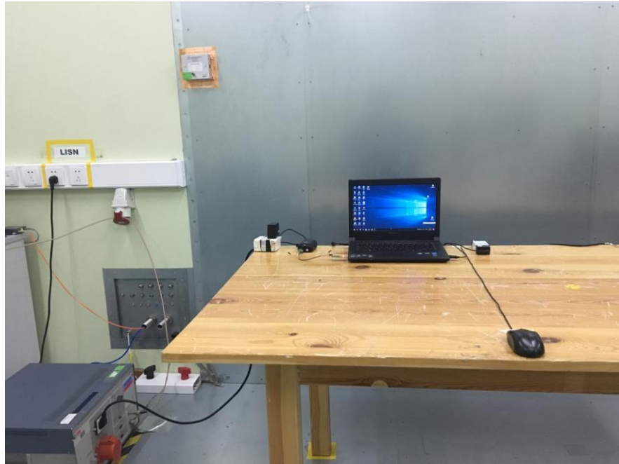
Figure 3: Conducted Emission Test Setup
