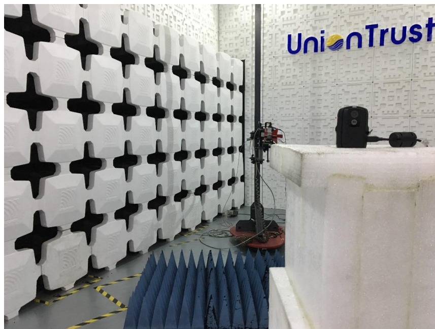
Figure 2: Radiated Emission Test Setup (Above 1GHz)
