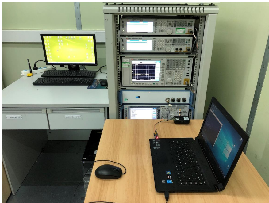
Figure 4: RF Conducted Test Setup
