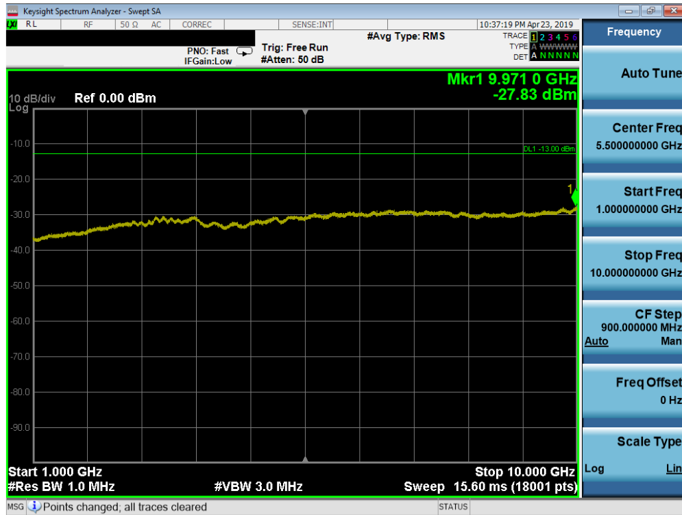
Plot 7-7. Conducted Spurious Plot (LTE Band 14, 10.0 MHz QPSK – RB Size 1, RB Offset 0 – Mid Channel)
