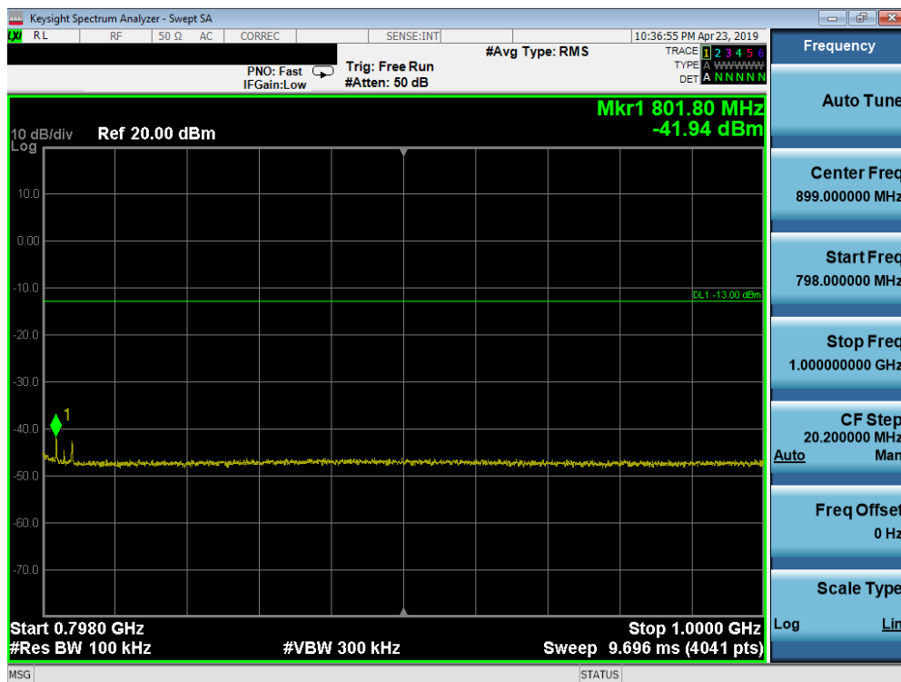
Plot 7-6. Conducted Spurious Plot (LTE Band 14, 10.0 MHz QPSK – RB Size 1, RB Offset 0 – Mid Channel)
