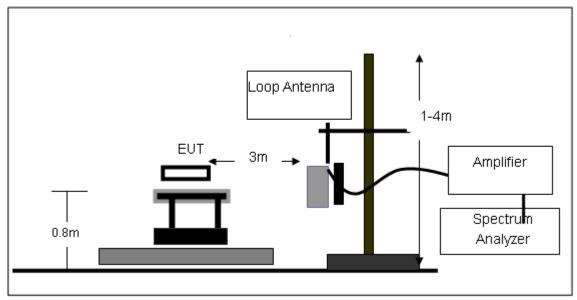
(B) Radiated Emission Test-Up Frequency 30MHz~1GHz
