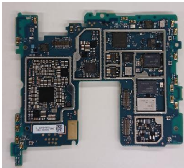
Internal PWB without Shield cases (Rear-side)
