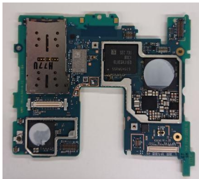
Internal PWB without Shield cases (Front-side)
